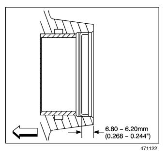
22. Install a NEW camshaft rear bearing hole plug to the proper depth.
