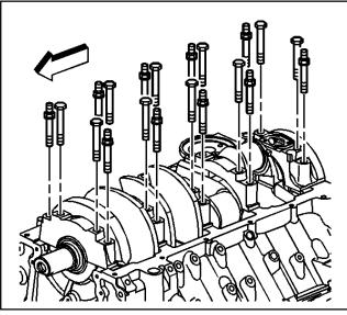
**Important:** Crankshaft bearing caps are machined with the engine block for the proper clearances. Mark or identify each crankshaft bearing cap location and direction before removal. Crankshaft bearing caps must be installed in their original locations.
