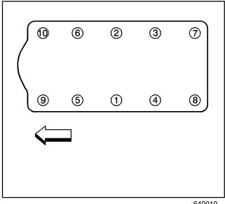
Important: The entire intake manifold tightening sequence must be followed exactly, or an oil leak resulting in engine damage may occur. Ensure the intake manifold is tightened without allowing the intake manifold to shift.
