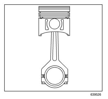
11. Inspect the connecting rod for an out-of-round bearing bore.
