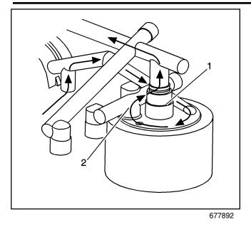
If both the oil filter and the oil cooler are plugged, the pressurized oil is routed around the top of the oil filter, through the oil filter bypass valve (2), through the oil cooler bypass valve (1) and directly into the engine oil passages. Lubrication still occurs, but the oil is not filtered or directed through the oil cooler.
