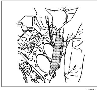
Inspect the engine block cylinder head deck for flatness using a straight edge and a feeler gauge.
