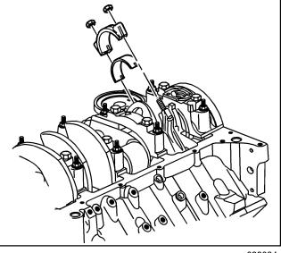
6. On the edge of the gauging plastic envelope, there is a graduated scale. Without removing the gauging plastic, measure the compressed width at the widest point.
