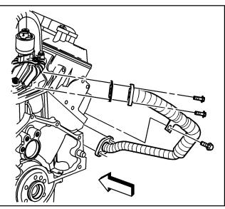
2. Remove the Exhaust Gas Recirculation (EGR) pipe bolts from the EGR adapter plate.
