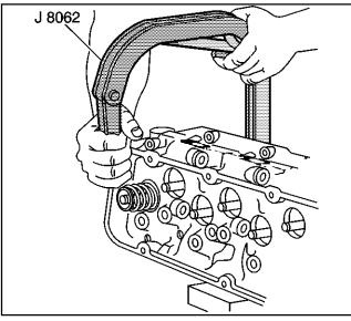
**Important:** When installing valve stem oil seals onto the valve guides, be careful not to tear the seal lip.
