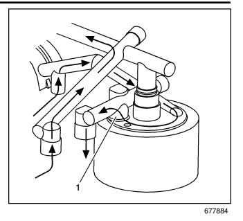
If the oil filter becomes plugged, the pressurized oil is diverted around the top of the oil filter. The oil filter bypass valve (1) is forced open, allowing the oil to continue on to the oil cooler and engine oil passages. No oil filteration occurs because the oil is not allowed into the oil filter.
