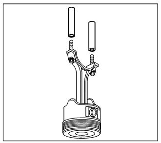
4. Install rubber fuel line onto the connecting rod bolts.
