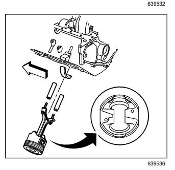
**Important:** The mark on the top of the piston must face the front of the engine block. When assembled, the flanges on the connecting rod and cap should face to the front of the block on the left bank and to the rear of the block on the right bank.
