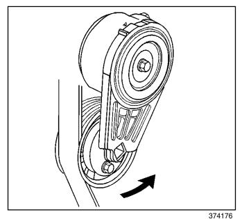
*Notice:* Allowing the drive belt tensioner to snap into the free position may result in damage to the tensioner.
