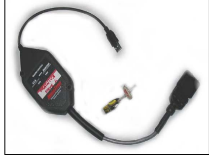
Figure 34. KVaser Communication Adapter
