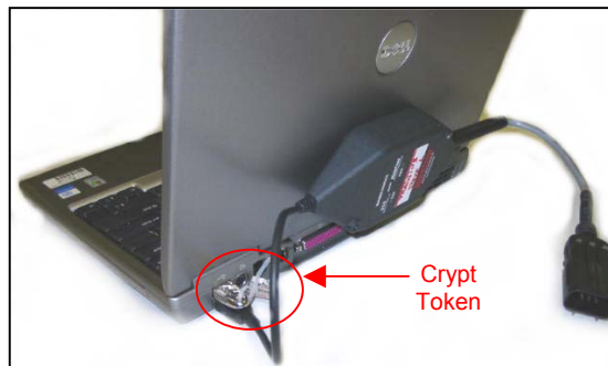
Figure 35. Crypt Token Installed on Laptop
