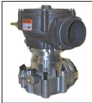
Figure 8. CA100 Mixer Attached to Throttle Body
