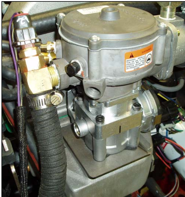
Figure 11. CA100 Mixer Installed with Electronic Throttle
