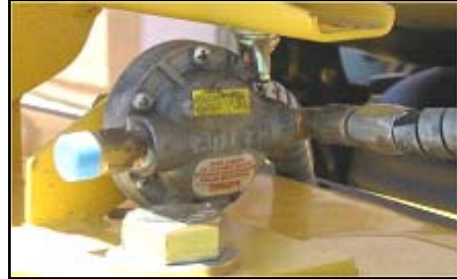
Figure 3. Inline LP Fuel Filter
