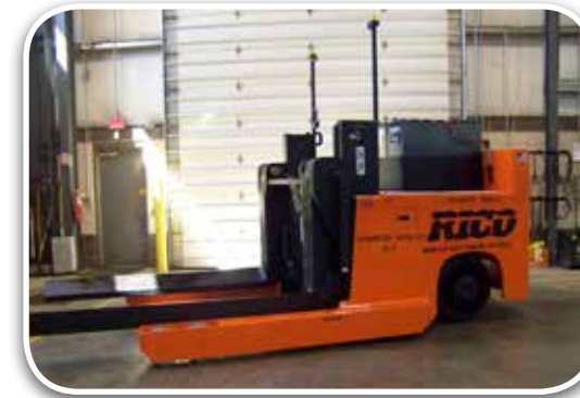
Remote Controlled Straddle
