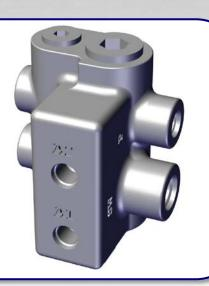
**2. Brake Valve Inching:** This inching pedal valve is for moving the truck in a slower more controlled speed. While you have the pedal pressed completely, the clutch plates in the transmission are disengaged so the truck will not move under power. As you lift the pedal the plates slowly engage giving controlled amounts of power to inch forward. Rico part # 33004205.
