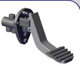
**5. Junction Block Assembly:** This junction block houses the brake switch and a test pressure port. The pressure port can be used during trouble shooting of the service brakes. Rico part # 5060990050-11
