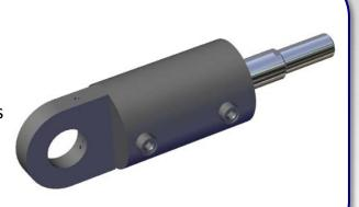
**8. Free Lift Cylinder:** "If equipped" the free lift cylinder is single acting and raises the inner mast without the inner mast raising beyond the top plain of the mast assembly. When the inner mast is raised beyond the top plain of the mast assembly the main lift cylinders take over. The free lift cylinder is part of the mast assembly. Part #'s vary between masts.
