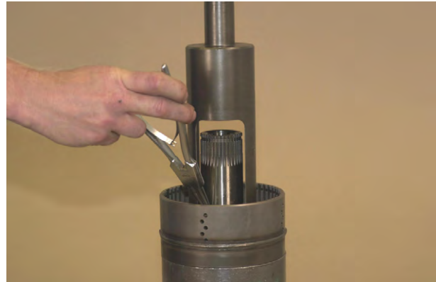
Figure 184 Compress spring and spring retainer and install spring retainer retaining ring.
