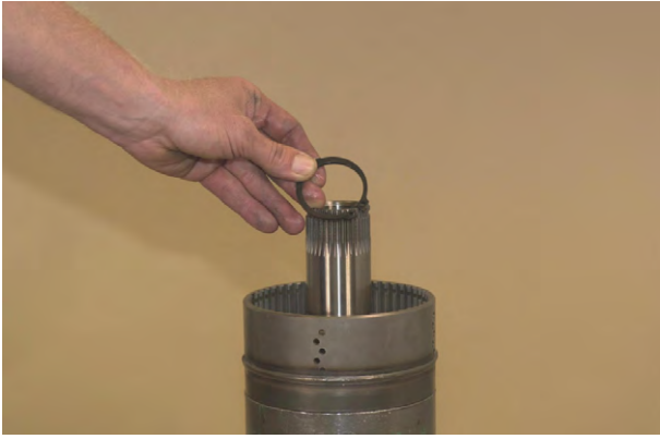
Figure 175 Remove inner bearing locating ring.
