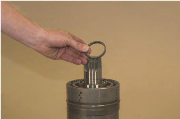
Figure 170 Remove low speed gear bearing spacer.
