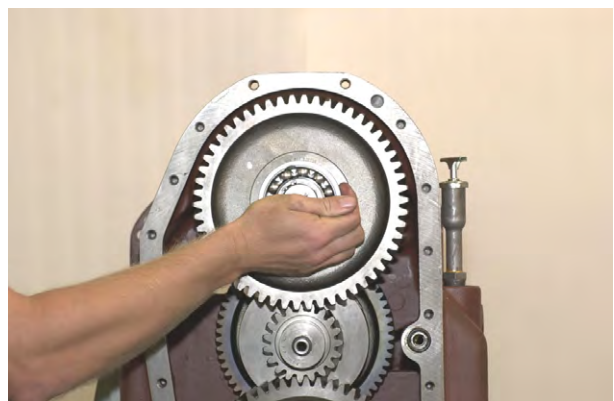
Figure 242 Position 3rd speed clutch assembly in pilot bearing. Use caution not to damage pilot bearing.
