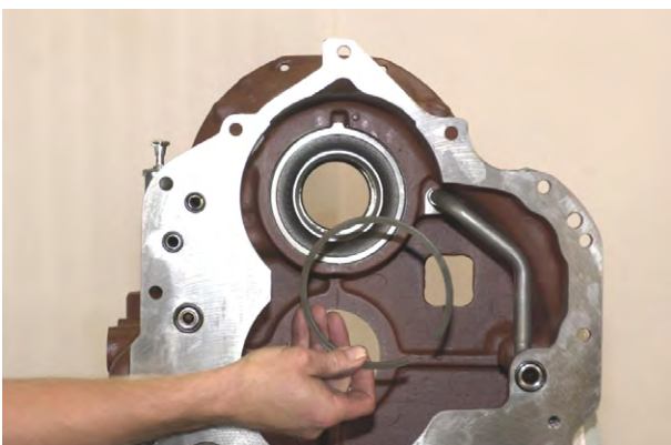
Figure 57 Remove forward clutch oil sealing ring sleeve retaining ring.
