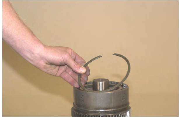
Figure 144 Install end plate retainer ring.
