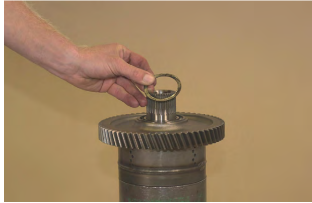
Figure 194 Position low gear front bearing spacer.
