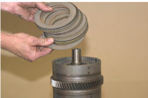
Figure 98 Remove inner and outer clutch discs.
