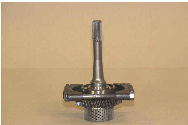
Figure 82 Remove turbine shaft bearing.
