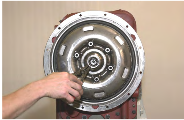
Figure 286 Install converter assembly retaining ring.
