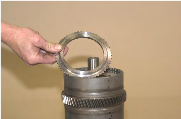
Figure 97 Remove end plate.
