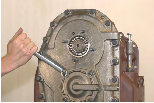
Figure 37 Remove low clutch shaft rear bearing cap nuts and lockwashers.
