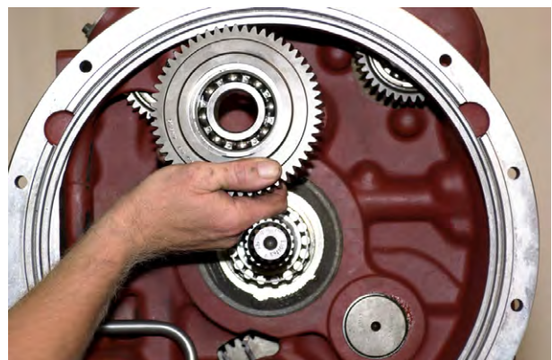
Figure 281 Position pump idler gear and bearing.
