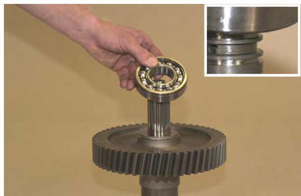
Figure 208 Install output shaft rear bearing. Note: Rear bearing locating ring groove must be up.
