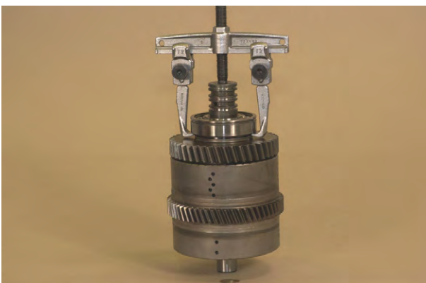
Figure 85 Remove clutch shaft front bearing.
