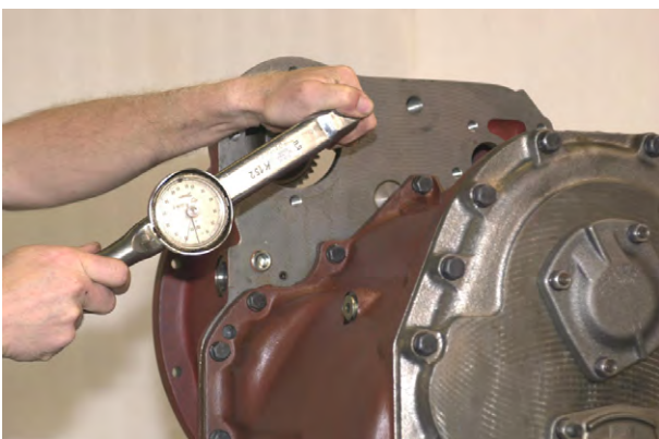
Figure 272 Install cap screw with Loctite® 243. Tighten cap screws 80-88 Ft.Lbs. [108-119Nm].
