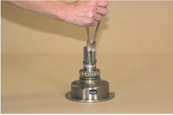
Figure 78 Remove stator support bearing retaining ring.
