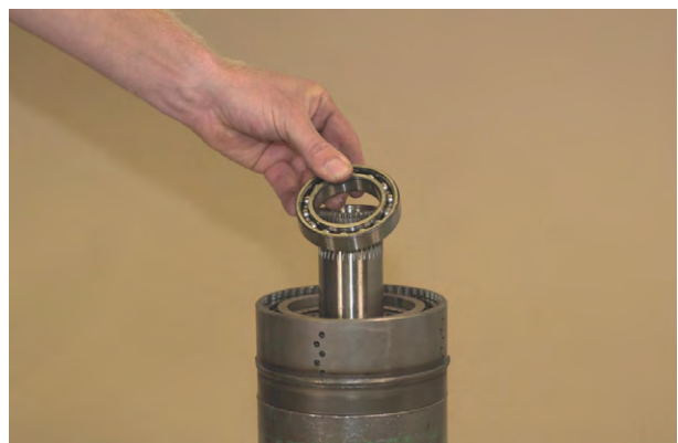
Figure 190 Install low speed gear inner bearing.
