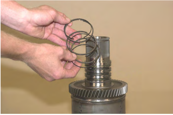
Figure 128 Remove clutch shaft sealing rings.
