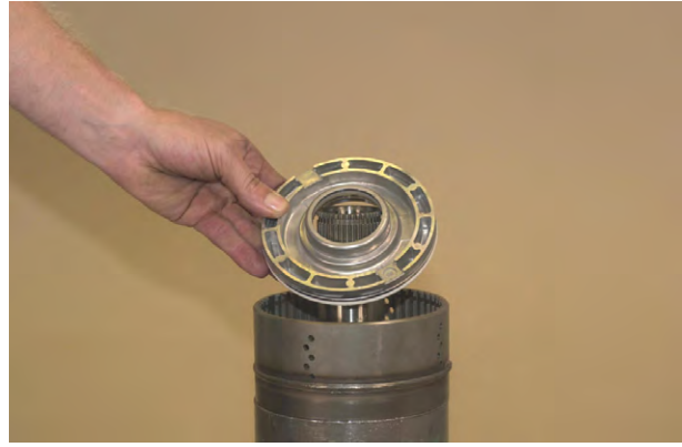
Figure 178 Remove clutch piston.
