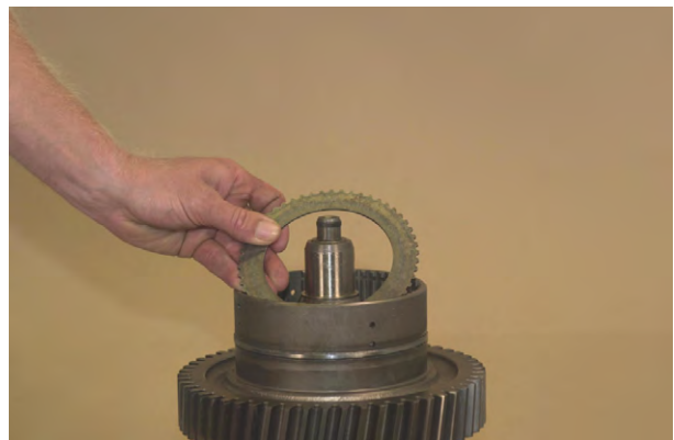
Figure 161 Install one (1) steel disc.
