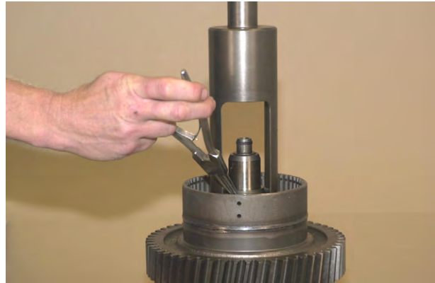
Figure 150 Compress piston return spring and spring retainer. Remove retainer ring.
