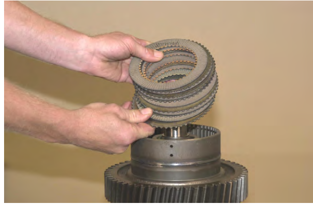
Figure 149 Remove inner and outer clutch discs.
