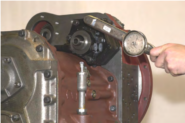
Figure 277 Tighten screws to specified torque. (See torque chart).
