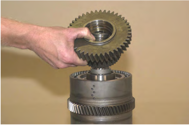
Figure 123 Install reverse gear into clutch drum. Align splines in reverse gear with internal teeth of friction discs.
