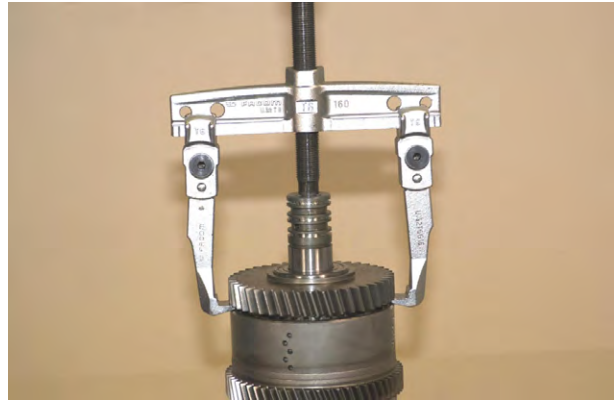
Figure 87 Remove reverse clutch gear and outer bearing.
