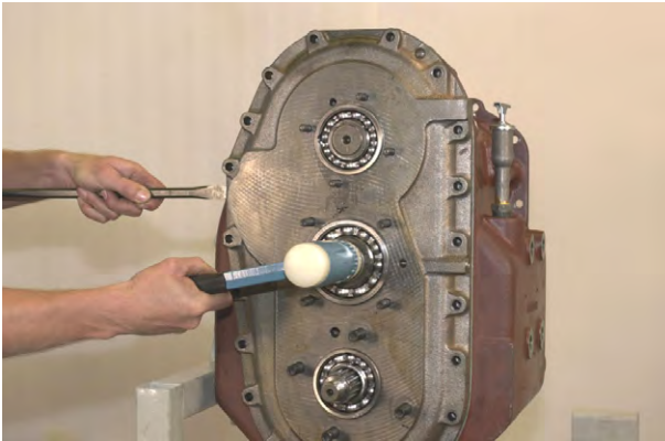
Figure 44 Using pry slots provided, pry cover from transmission housing. Tapping on clutch and output shaft will allow cover to be removed without shafts bending. Note: The use of alignment studs will facilitate cover removal.
