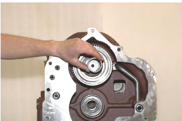
Figure 262 Position pilot bearing on forward clutch shaft.
