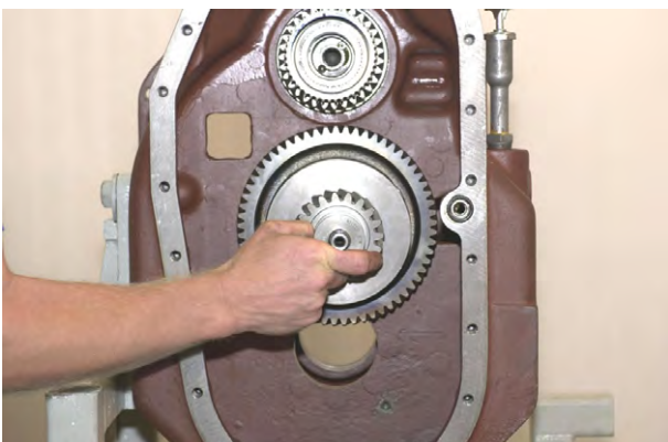
Figure 239 Locate low clutch assembly in housing. Tap into position.
