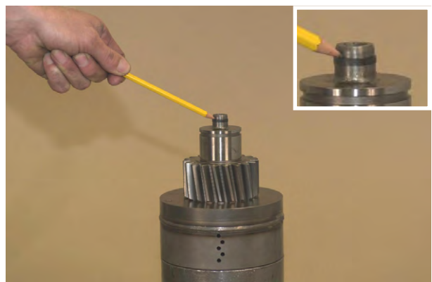
Figure 196 Install new oil seal ring on low clutch shaft.
