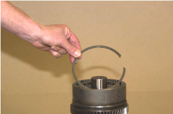
Figure 129 Remove end plate retainer ring.
