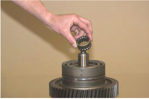
Figure 146 Remove clutch shaft pilot bearing.
