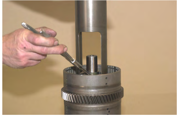
Figure 99 Compress piston return spring and remove retainer ring.
