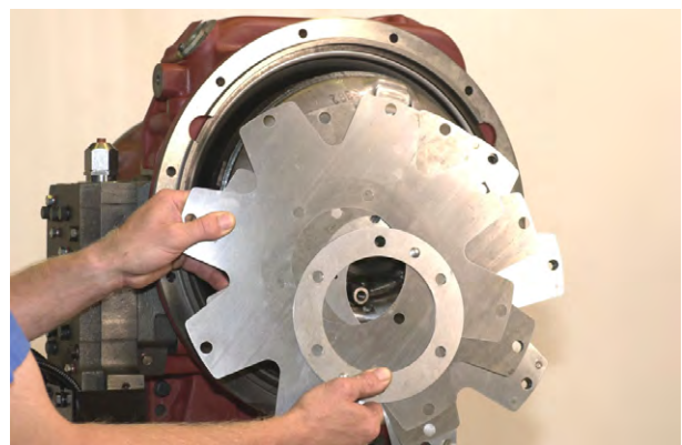
Figure 6 Remove drive plates and backing ring.
