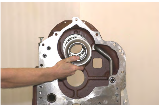
Figure 233 Tap forward shaft piston ring sleeve into position.
