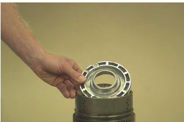
Figure 137 Install clutch piston in clutch drum. Use caution not to damage sealing rings.
