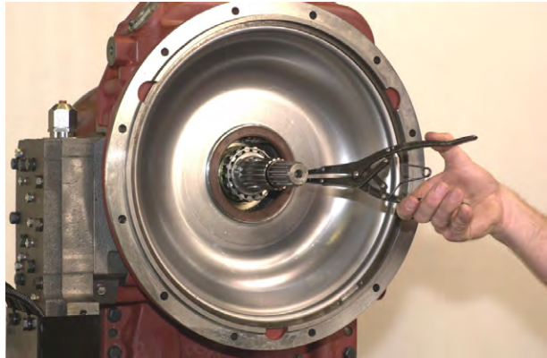
Figure 11 Remove turbine locating ring.
