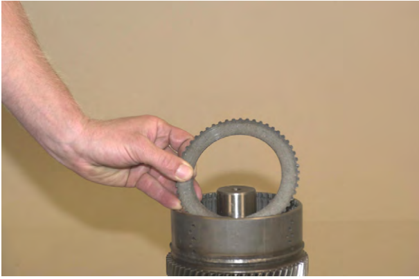
Figure 141 Install one (1) steel disc.
