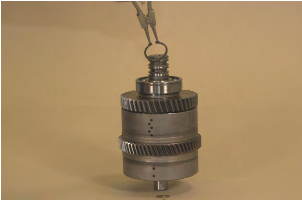
Figure 84 Remove clutch shaft front bearing retaining ring.
