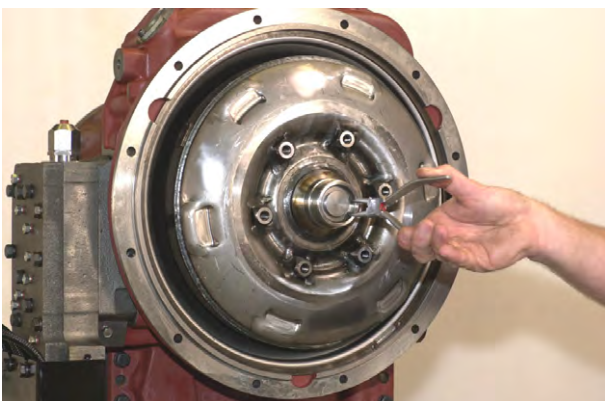
Figure 9 Through the bore plug hole, remove turbine retaining ring.
