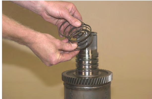
Figure 145 Install clutch shaft sealing rings.
