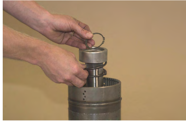
Figure 183 Position piston retainer spring, spring retainer and snap ring in clutch drum.
