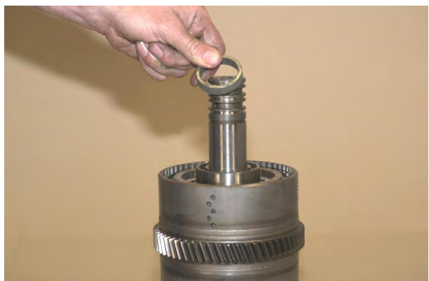
Figure 122 Install clutch gear bearing spacer.
