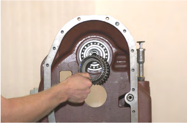
Figure 237 From the rear locate 3rd gear and clutch disc hub on forward shaft.
