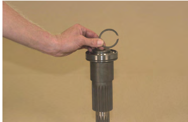
Figure 201 Remove output shaft front bearing retaining ring.
