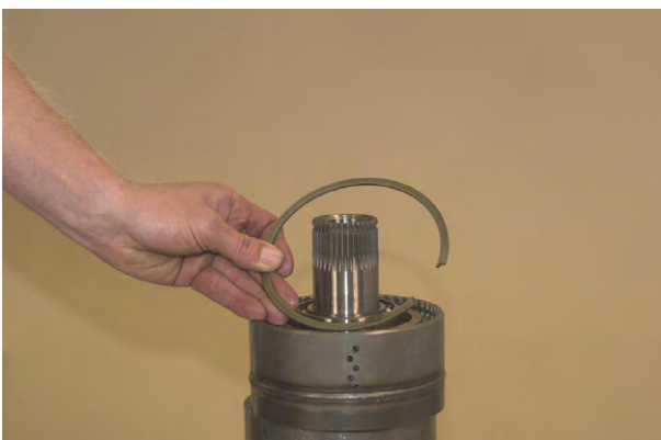
Figure 171 Remove end plate retaining ring.
