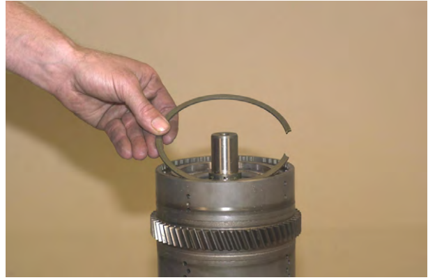
Figure 110 Install end plate retainer ring.
