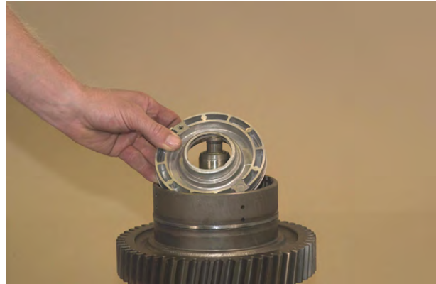
Figure 160 Install clutch piston in clutch drum. Use caution as not to damage sealing rings.
