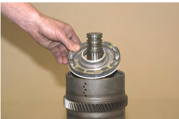
Figure 113 Install clutch piston in clutch drum. Use caution not to damage sealing rings.
