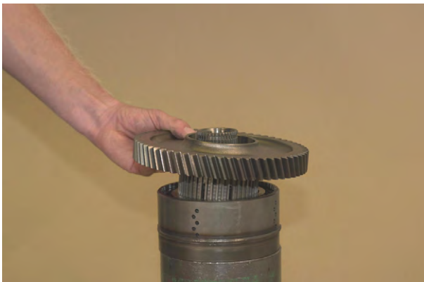
Figure 192 Install clutch driven gear and hub into the clutch drum. Align splines on the clutch hub with the internal teeth of the friction discs. Tap gear into position. DO NOT FORCE THIS OPERATION. Gear splines must be in full position with internal teeth of all the friction discs.
