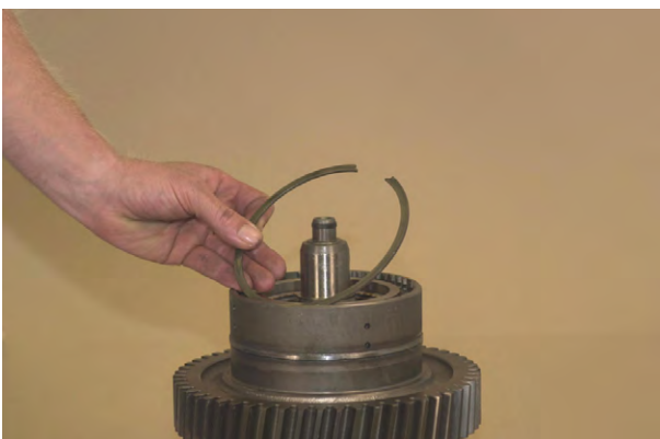
Figure 164 Install end plate retaining ring.
