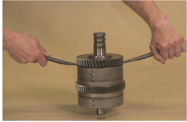
Figure 86 Pry reverse gear from clutch assembly far enough to use a gear puller.
