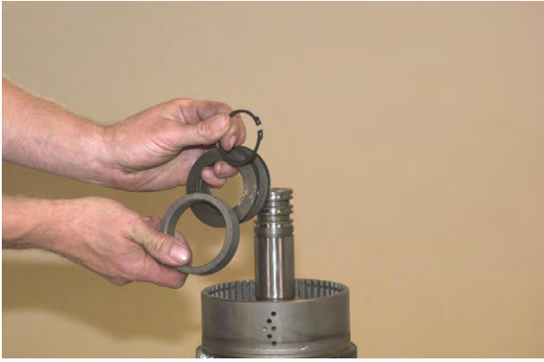
Figure 94 Remove piston disc springs and piston spacer.
