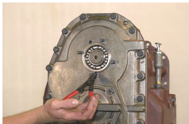
Figure 36 Remove 3rd shaft rear bearing locating ring.
