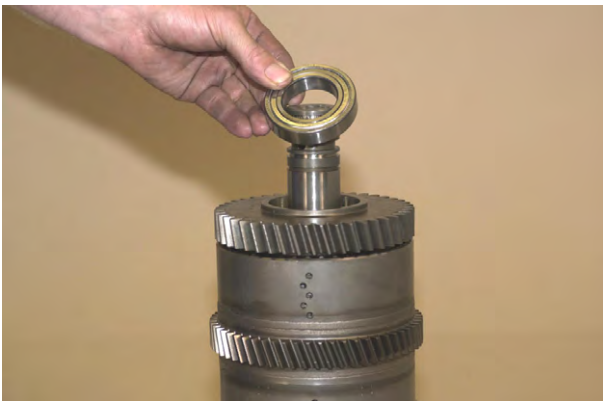
Figure 124 Install clutch gear outer bearing.
