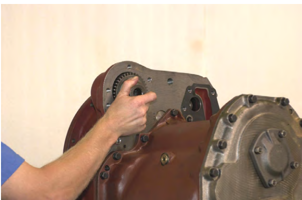
Figure 21 Remove auxiliary pump drive gear.
