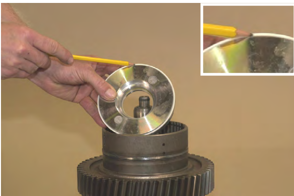
Figure 158 Refer to the "Cleaning and Inspection" pages. The bleed valve in the clutch piston must be clean and free from any foreign material. Install clutch piston outer seal ring. Size as described in figure 102.
