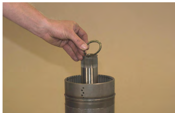
Figure 185 Install clutch inner bearing locating ring.
