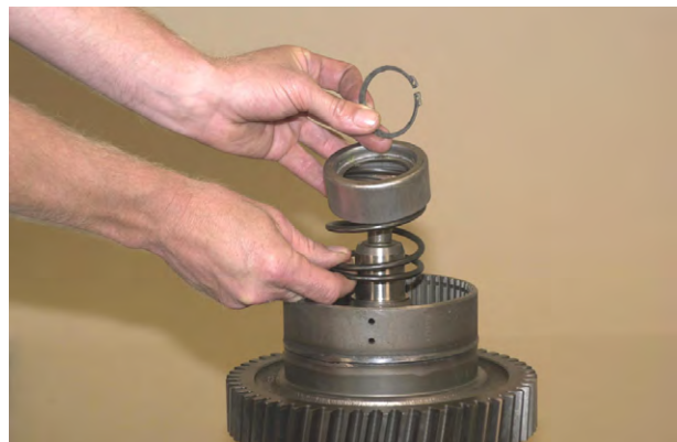
Figure 151 Remove return spring, spring retainer and retainer ring.
