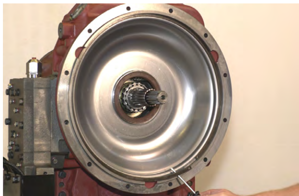
Figure 12 Using slots provided in converter housing, remove oil baffle retaining ring.
