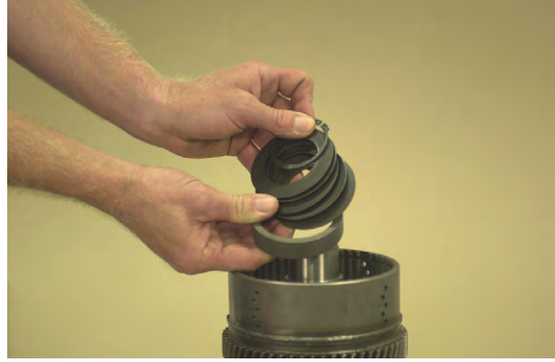
Figure 138 Position spring spacer, piston return springs and retainer ring. First spring with large diameter towards spacer. See figure 139. Alternate five (5) springs. See note figure 94.
