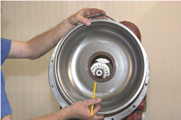
Figure 283 Press new seal in baffle with lip of seal towards impeller hub bearing. Position new sealing ring on oil baffle.
