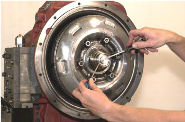
Figure 8 Using 2 small screwdrivers as shown, remove bore plug.
