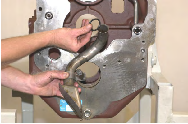
Figure 61 Remove suction tube and "O" ring.
