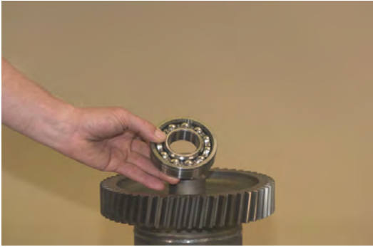
Figure 156 Refer to the "Cleaning and Inspection" pages. Install 3rd clutch shaft rear bearing.
