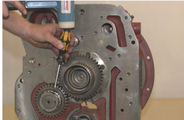
Figure 229 Bend over tag of lock plate which aligns with one of the slots of the lock nut to secure it. See figure 230.
