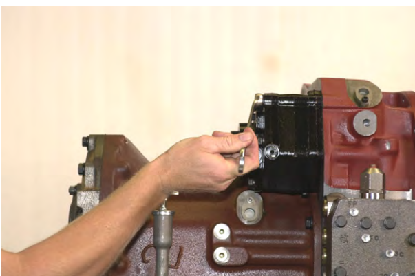
Figure 3 Remove pressure regulating valve and charging pump bolts.
