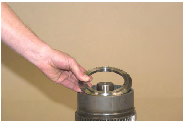
Figure 130 Remove end plate.
