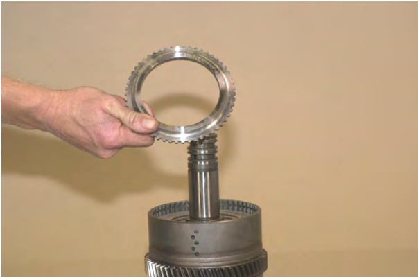
Figure 90 Remove end plate.
