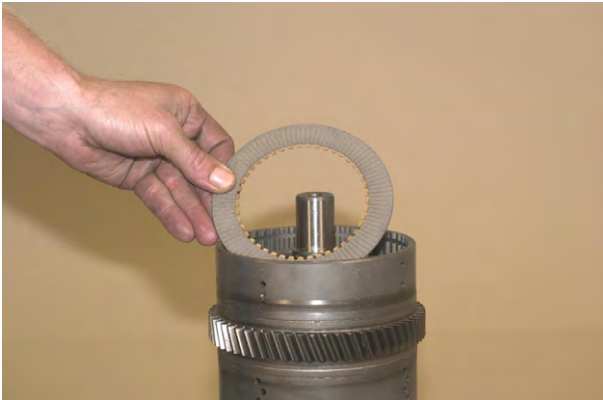
Figure 108 Install one friction disc. Alternate steel and friction discs until the proper amount of discs are installed. First disc next to piston is steel, last disc installed is friction.
