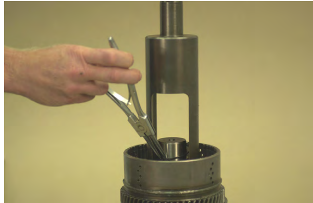
Figure 132 Compress piston return disc springs and remove retainer ring.
