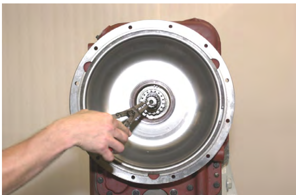
Figure 284 Position oil baffle in housing and install retaining ring. Make certain ring is in full position in ring groove.
