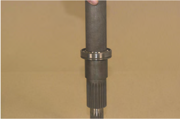
Figure 203 Tap front bearing into place.
