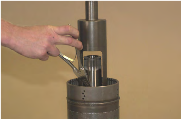
Figure 176 Compress piston return spring and spring retainer. Remove retainer ring.
