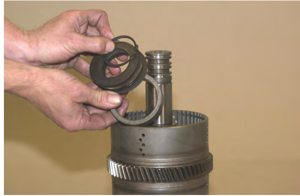
Figure 114 Position spring spacer and piston return spring with large diameter towards spacer. (See figure 115). Alternate five (5) springs, see note figure 94.
