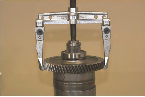
Figure 169 Remove low gear and hub, low shaft front bearing, bearing spacer and clutch gear outer bearing.
