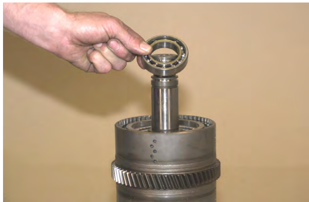
Figure 121 Install clutch gear inner bearing. Note: This bearing does not have a shield in it.
