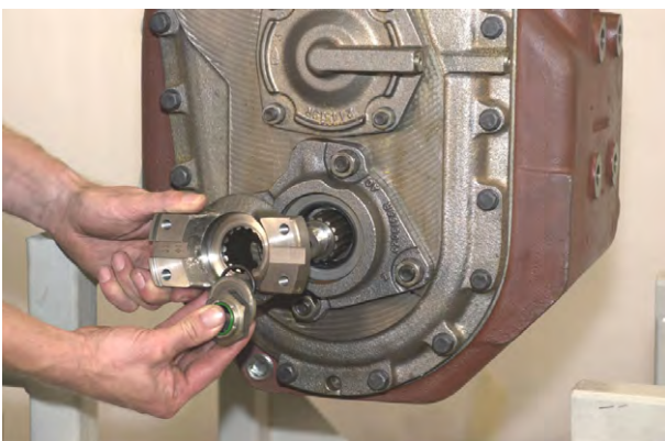
Figure 33 Output flange, "O" ring, washer and nut removed.
