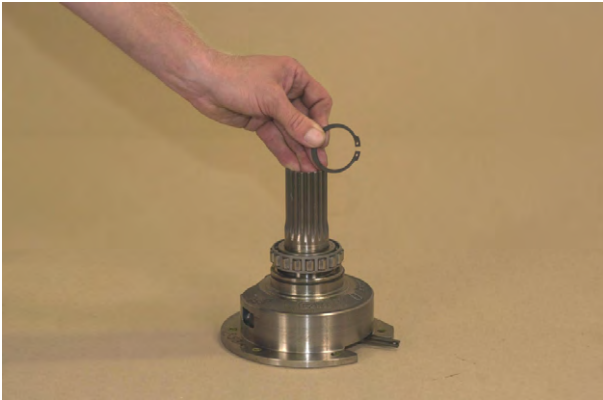
Figure 213 Install bearing retaining ring.
