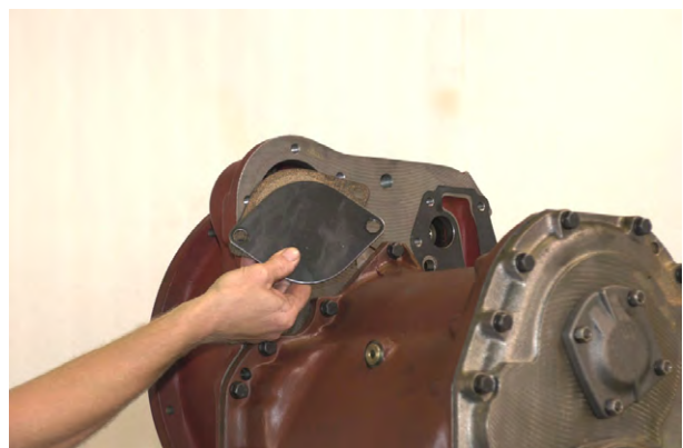
Figure 18 Remove pump hole cover and gasket.
