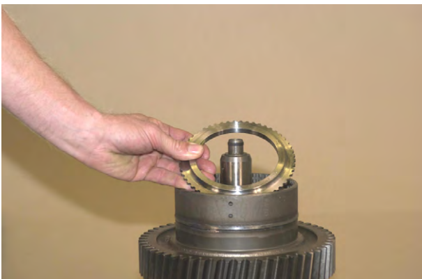
Figure 148 Remove end plate.
