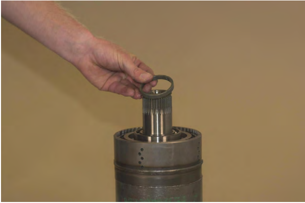
Figure 191 Install low speed gear bearing spacer.
