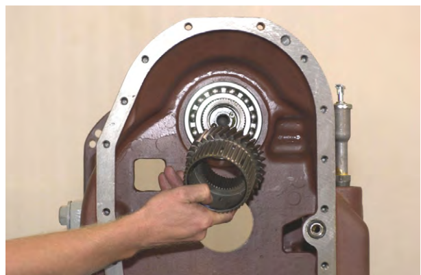
Figure 54 Remove 3rd clutch disc hub.
