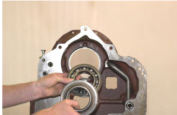
Figure 59 Sleeve and bearing removed.
