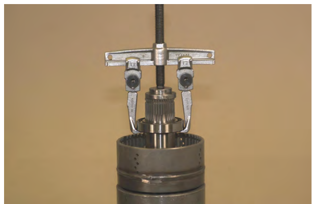
Figure 174 Remove low speed gear inner bearing.
