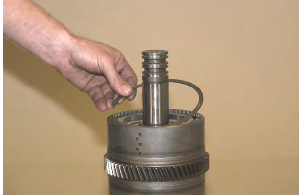
Figure 120 Install end plate retaining ring.
