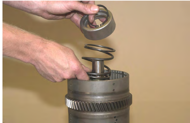
Figure 100 Remove return spring, spring retainer and retainer ring.
