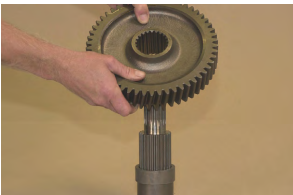
Figure 199 Remove output shaft gear.
