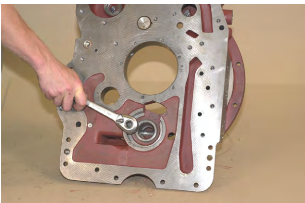
Figure 76 Remove oil sealing ring sleeve retainer screw and lockwasher. Remove sleeve lock.
