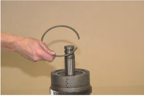
Figure 89 Remove end plate retaining ring.
