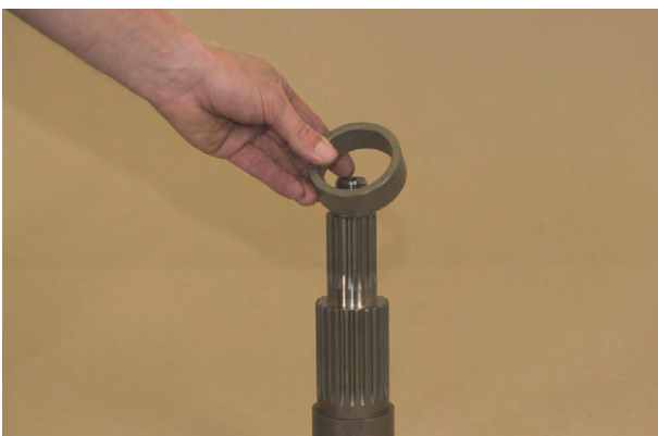
Figure 205 Position output shaft gear spacer.
