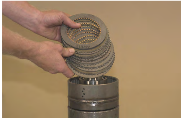
Figure 173 Remove inner and outer clutch discs. Do not mix low clutch friction discs with friction discs in other clutches.
