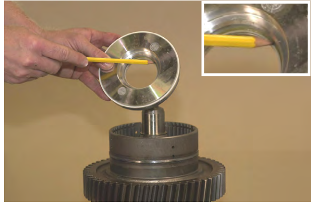
Figure 159 Install clutch piston inner seal ring. Size sealing ring as described in figure 102.
