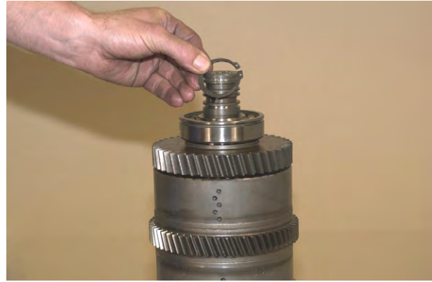
Figure 126 Install bearing retainer ring.
