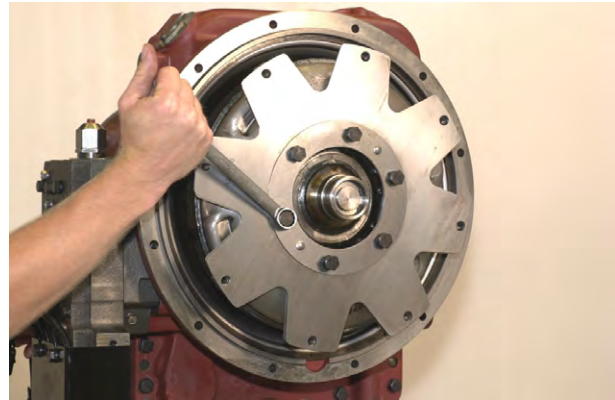
Figure 5 Remove drive plate mounting screws and lockwashers.
