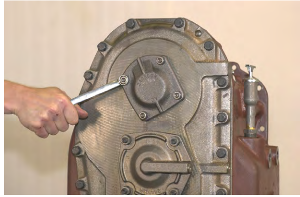
Figure 34 Remove 3rd speed clutch rear bearing cap stud nuts and lockwashers.
