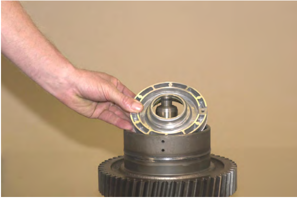
Figure 152 Remove clutch piston.
