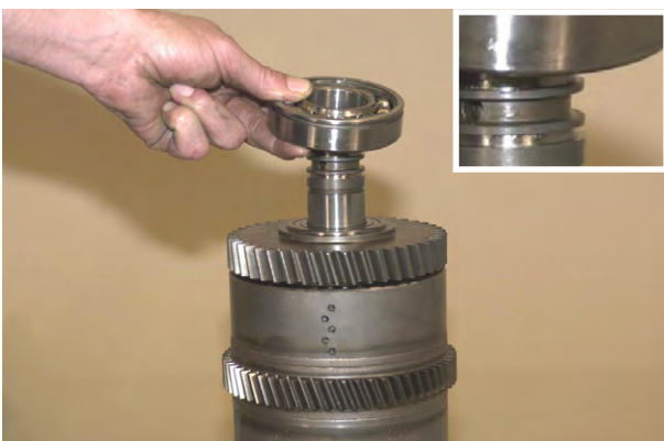
Figure 125 Install clutch shaft front bearing.
