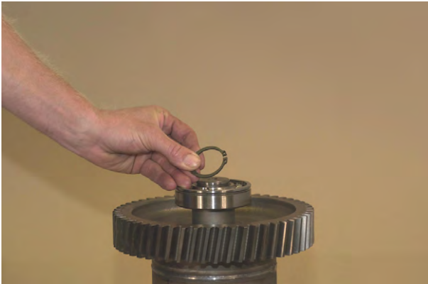
Figure 157 Install rear bearing retaining ring.
