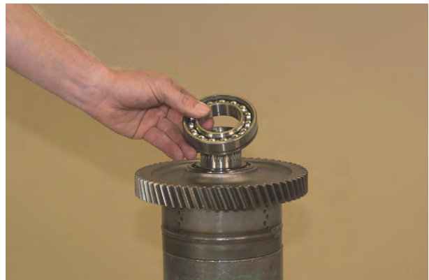
Figure 195 Install low clutch shaft front bearing.
