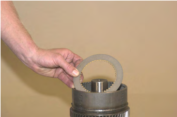
Figure 142 Install one (1) friction disc. Alternate steel and friction discs until proper amount of discs are installed. First disc next to piston is steel, last disc installed is friction.
