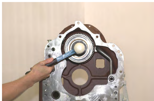
Figure 236 Tap clutch assembly into position.
