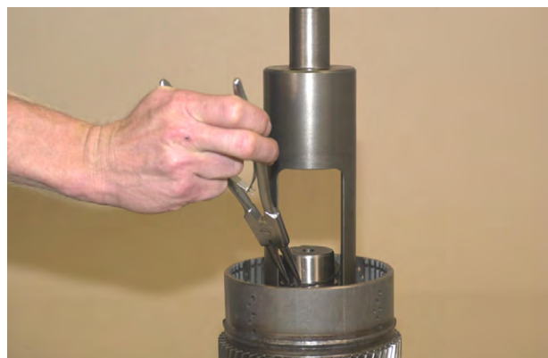
Figure 140 Compress piston return disc springs and install return spring retainer ring.
