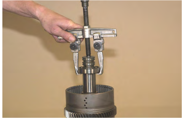
Figure 92 Remove clutch gear inner bearing.
