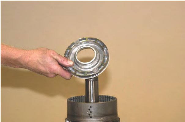
Figure 95 Remove clutch piston.
