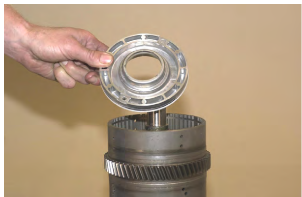
Figure 101 Remove clutch piston.
