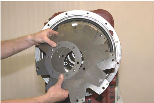
Figure 289 See special section on page 5-1 for drive plate installation.
