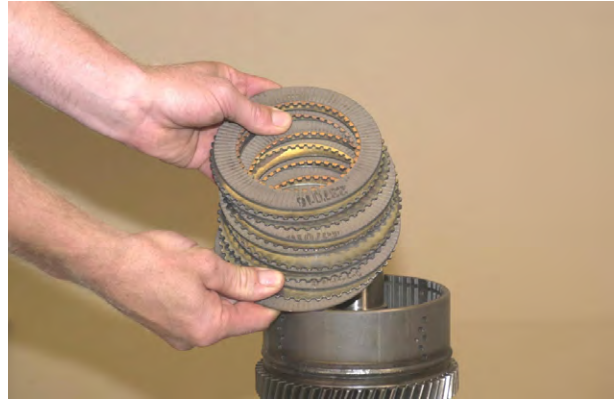
Figure 131 Remove inner and outer clutch discs.
