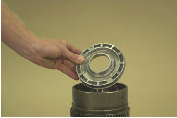
Figure 134 Remove clutch piston.
