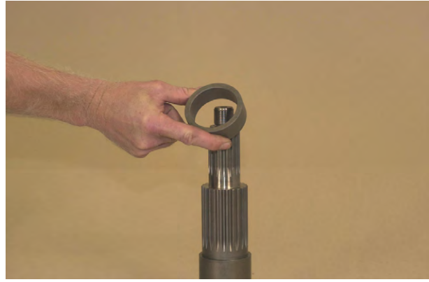
Figure 200 Remove output shaft gear spacer.
