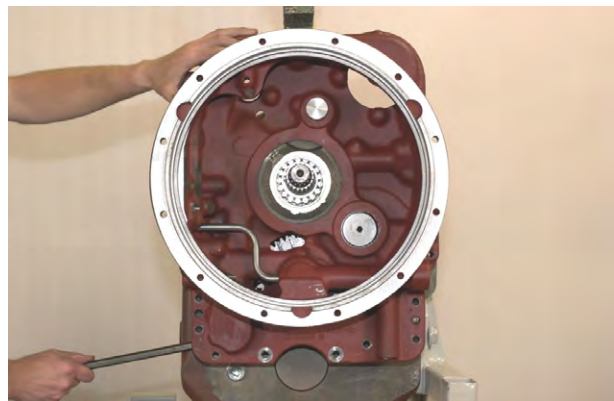
Figure 30 Support converter housing with a chain hoist. Remove remaining bolt and pry converter housing from transmission case.
