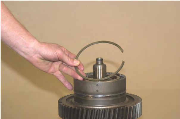
Figure 147 Remove end plate retaining ring.
