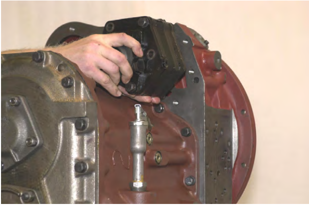
Figure 276 Using a new gasket and “O” ring, position charging pump assembly. Install cap screws and lockwashers.
