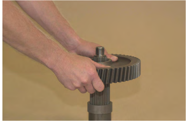
Figure 206 Install output gear (long hub down).
