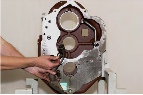
Figure 231 Install suction tube and new "O" ring.
