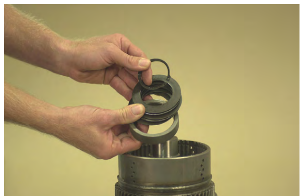
Figure 133 Remove piston return disc springs and piston spacer. See note figure 94.
