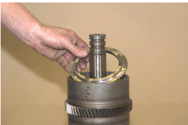
Figure 119 Install end plate.
