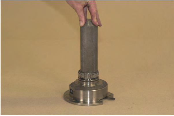
Figure 212 Press support bearing into position.
