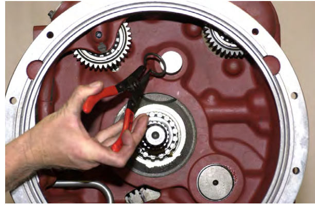
Figure 280 Install idler gear bearing retaining ring.
