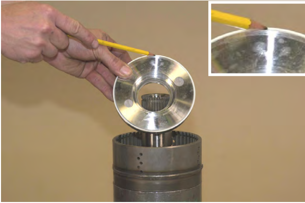
Figure 180 Refer to the "Cleaning and Inspection" pages. The bleed valve in the clutch drum must be clean and free of any foreign material. Install clutch piston outer seal. Size as described in figure 102.
