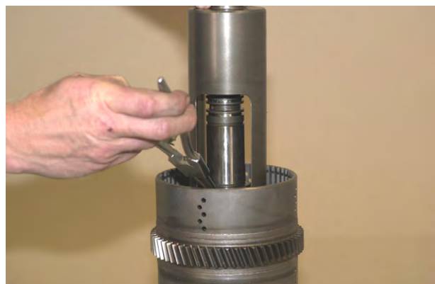
Figure 116 Position spring snapping. Compress spring and install snapping.
