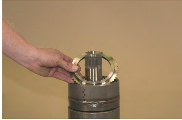
Figure 172 Remove end plate.
