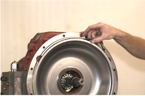
Figure 13 Baffle and sealing ring removed.
