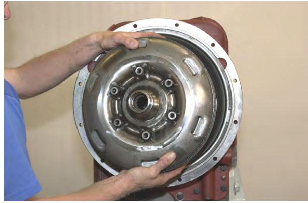
Figure 285 Position converter assembly on stator support and turbine shaft.
