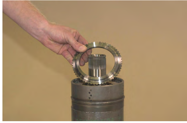
Figure 188 Install clutch disc end plate.
