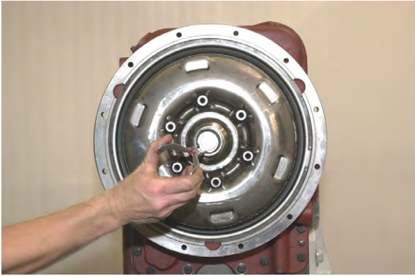
Figure 288 Install bore plug retaining ring.
