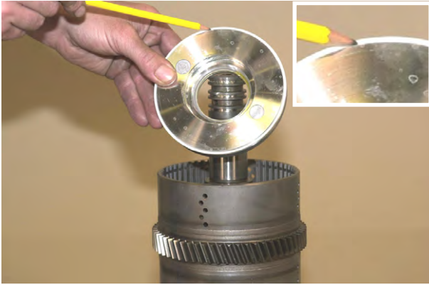
Figure 111 Refer to the "Cleaning and Inspection" pages. Install clutch piston outer seal ring. Size as described in figure 102.
