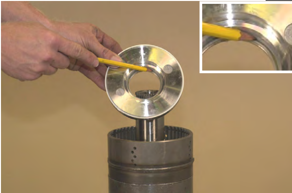
Figure 181 Install clutch piston inner seal ring and size as described in figure 102.
