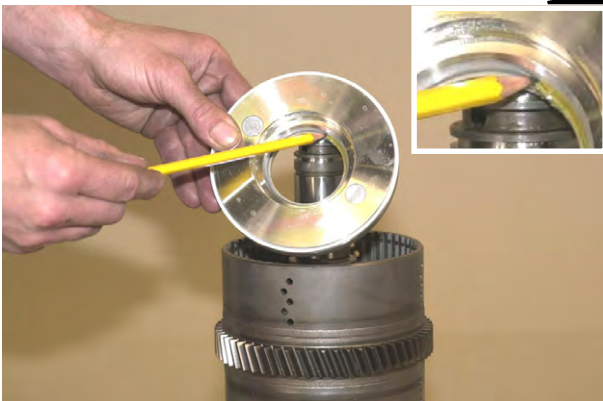
Figure 112 Install clutch piston inner seal ring. Size as described in figure 102.
