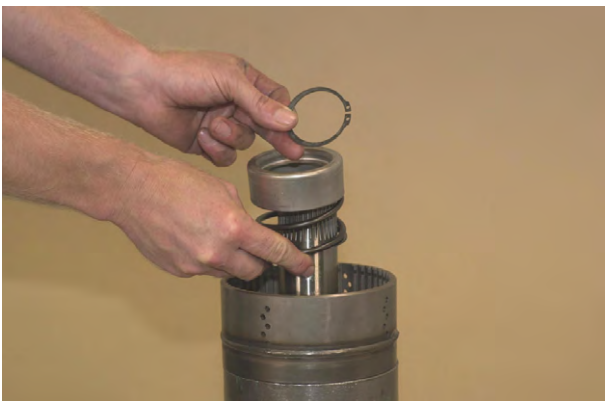
Figure 177 Remove spring retainer ring, spring retainer and spring.
