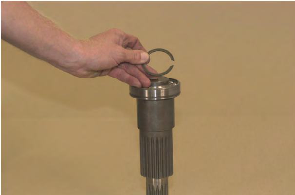
Figure 204 Install output shaft front bearing retaining ring.
