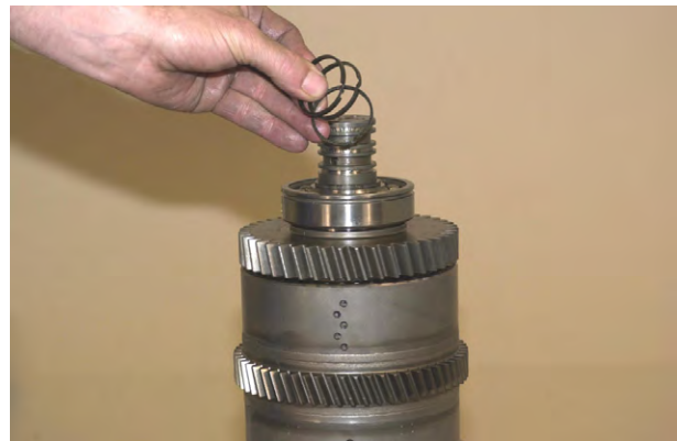
Figure 127 Install clutch shaft piston rings.
