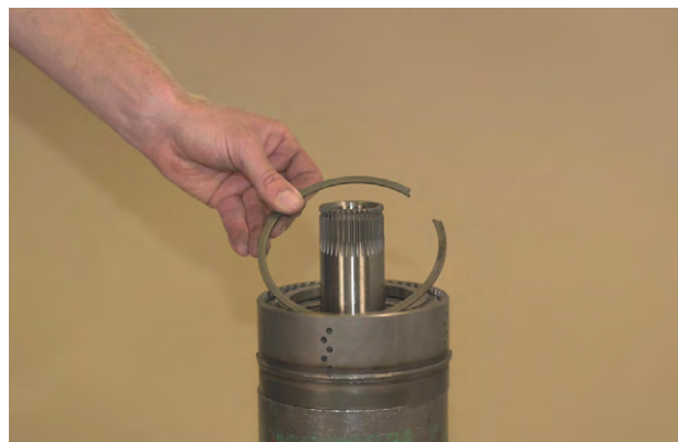
Figure 189 Install end plate retainer ring.
