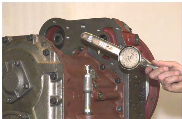
Figure 275 Install cap screws with Loctite® 243. Tighten cap screws 80-88 Ft.Lbs. [108-119Nm].
