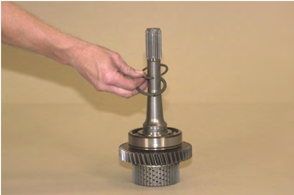
Figure 81 Remove turbine shaft bearing retaining ring and washer.
