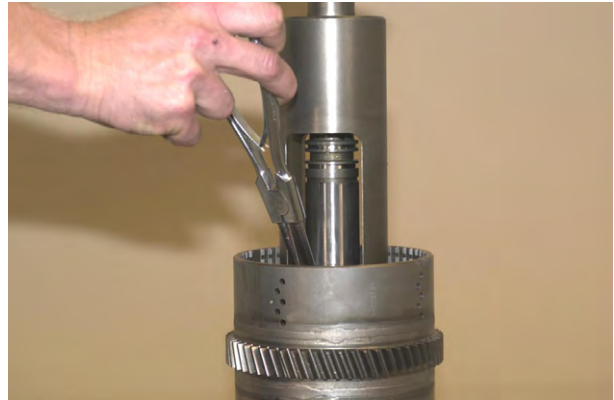
Figure 93 Compress spring and through opening remove spring retainer snap ring. Release tension on spring and remove clutch piston return spring. A sleeve with a portion removed is recommended for removing the clutch piston spring, washer and retainer ring.
