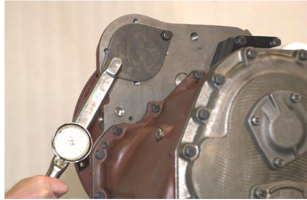
Figure 279 Install pump hole cover, new gasket, screws and lockwashers. Tighten screws to specified torque. (See torque chart).
