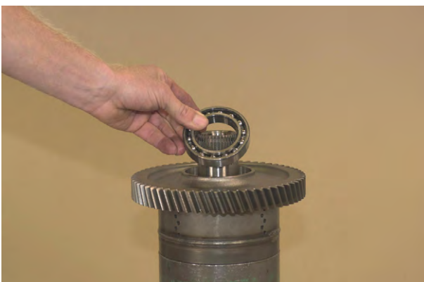
Figure 193 Install low speed gear outer bearing.
