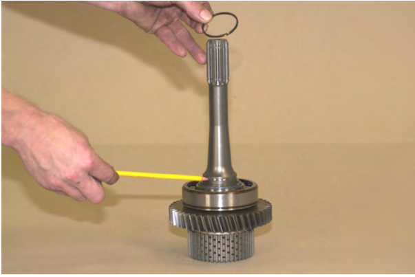
Figure 80 Remove turbine shaft oil sealing ring.
