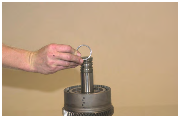
Figure 88 Remove clutch gear bearing spacer.
