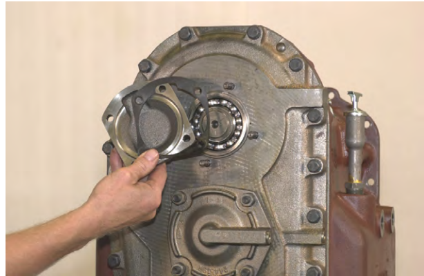
Figure 35 3rd shaft bearing cap and gasket removed.
