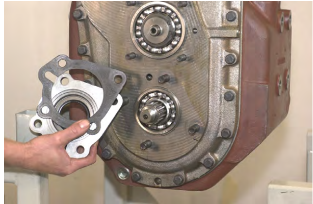
Figure 41 Remove output shaft bearing cap and gasket.
