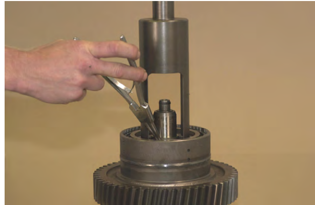
Figure 166 Compress return spring and install retaining ring.
