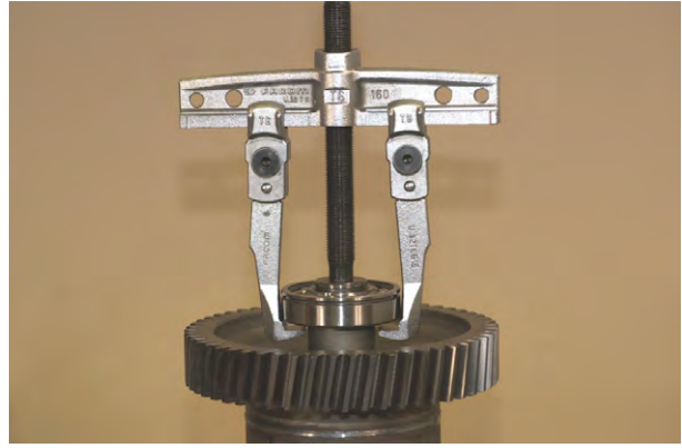
Figure 155 Remove 3rd clutch shaft rear bearing.
