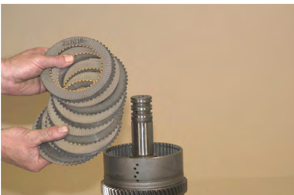
Figure 91 Remove inner and outer discs.
