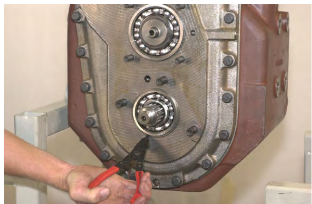
Figure 42 Remove output shaft rear bearing locating ring.
