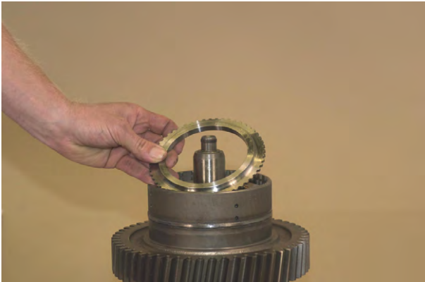
Figure 163 Install end plate.
