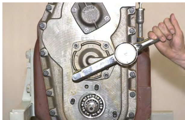
Figure 254 Install lockwashers and stud nuts. Tighten nuts to specified torque. (See torque chart).
