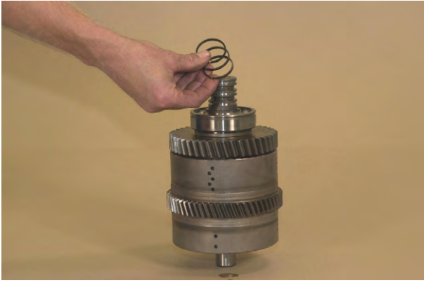
Figure 83 Remove clutch shaft piston rings.
