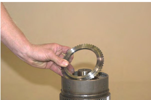
Figure 143 Install end plate.
