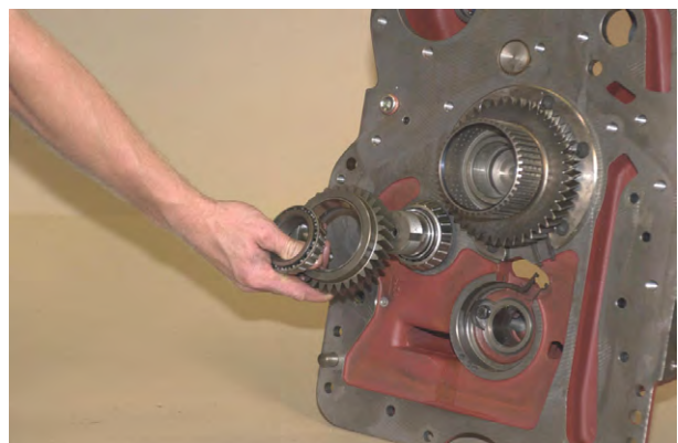
Figure 67 Outer taper bearing and idler gear removed.
