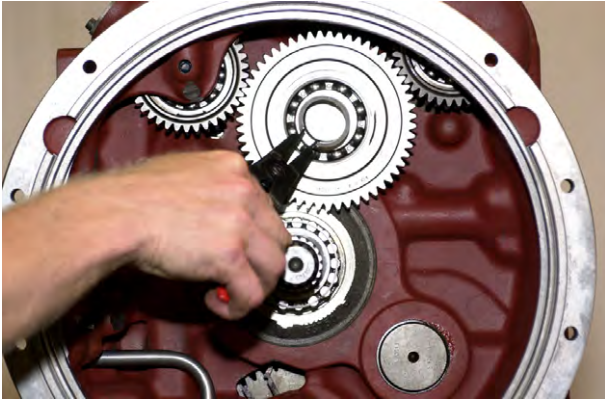
Figure 282 Install idler gear bearing locating ring.
