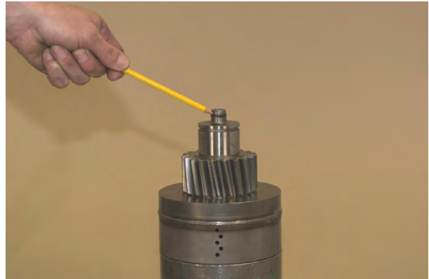
Figure 179 Remove clutch shaft piston ring.
