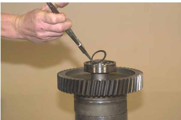
Figure 154 Remove 3rd clutch shaft rear bearing retaining ring.
