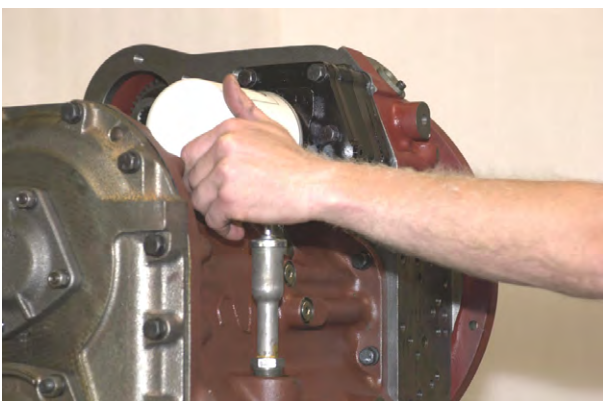
Figure 278 Install new oil filter. Tighten to 20-25 Ft.Lbs. [27.1-33.9Nm].
