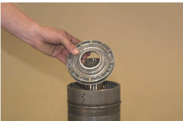
Figure 182 Position piston in clutch drum as shown. Use caution not to damage inner and outer piston seal rings.
