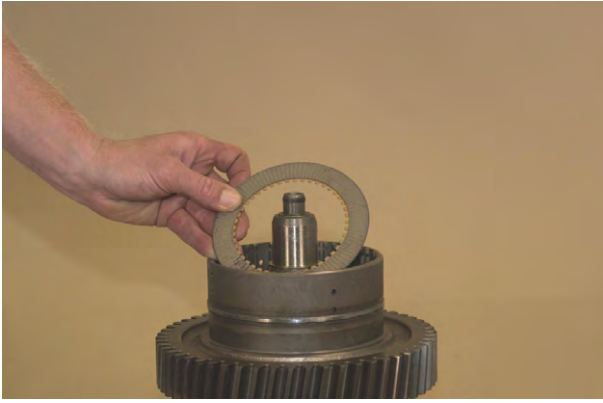
Figure 162 Install one (1) friction disc. Alternate steel and friction discs until the proper amount of discs are installed. First disc next to the piston is steel, last disc installed is friction.
