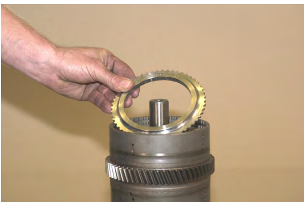
Figure 109 Install end plate.
