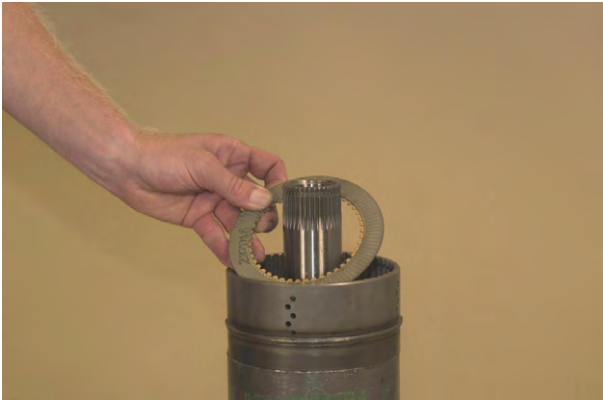
Figure 187 Install one friction disc. Alternate steel and friction discs until proper amount of discs are installed. First disc next to the piston is steel, last disc installed is friction.
