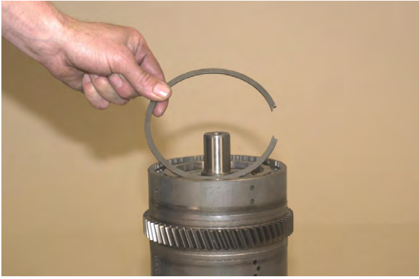
Figure 96 Remove end plate retaining ring.
