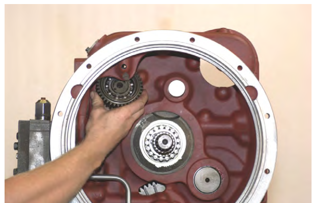
Figure 24 From the front, tap pump drive gear and bearing support from housing.
