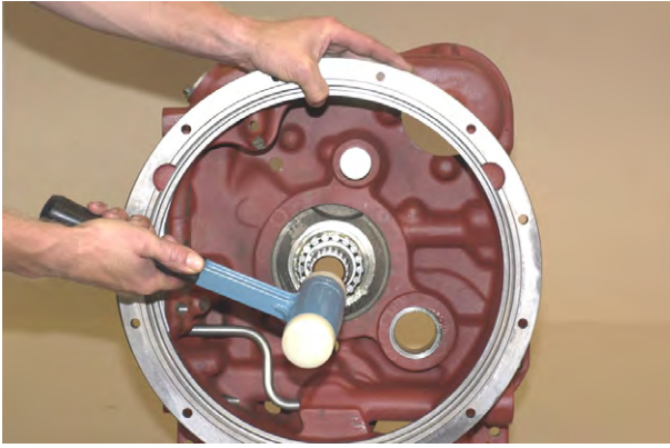
Figure 74 Tap stator support from converter housing.
