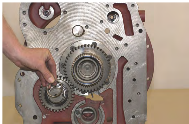
Figure 224 Position bearing spacer on shaft.
