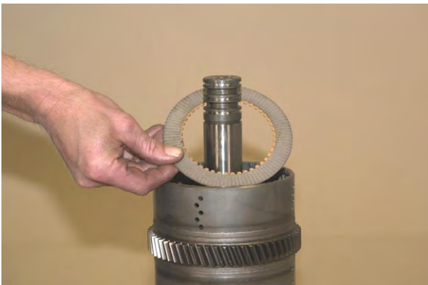
Figure 118 Install one (1) friction disc. Alternate steel and friction discs until proper amount of discs are installed. First disc next to the piston is steel, last disc installed is friction.
