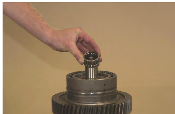
Figure 167 Install clutch shaft pilot bearing.
