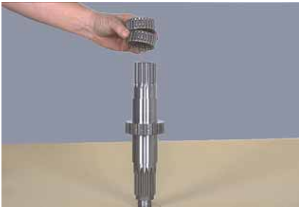
Figure 8 Remove high range gear bearings.
