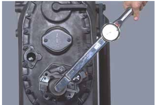
Figure 44 Block flange to prevent turning. Tighten flange nut to specified torque (see elastic stop nut chart).
