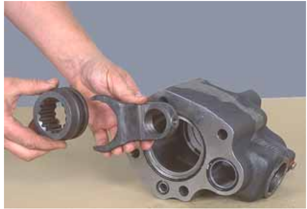
Figure 27 Shift and shift fork removed.
