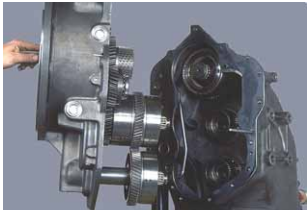
Figure 278 The use of two aligning studs will facilitate aligning the converter housing to the transmission housing. Install converter housing assembly to transmission assembly using extreme caution as to align the clutch pilots to clutch disc hubs. As the clutch pilots enter the disc hubs, turn the turbine shaft and output shaft back and forth. This will help align all of the clutch inner discs with the disc hubs. DO NOT FORCE THIS OPERATION. When all clutches are properly aligned, the converter housing will be tight against the transmission housing. Install two housing to housing capscrews and lockwashers. Remove aligning studs. Install remaining capscrews and lockwashers.
