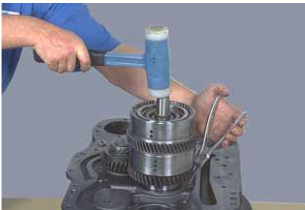
Figure 211 Spread ears on reverse clutch front bearing locating ring. Tap reverse and 2nd clutch assembly into converter housing. Align the snap ring groove in the bearing with the snap ring in the housing, being certain bearing snap ring is in full position in snap ring groove.
