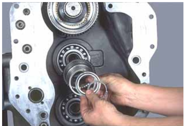
Figure 48 Remove 2nd clutch disc hub, retaining ring, retaining ring retainer and retainer locating ring.
