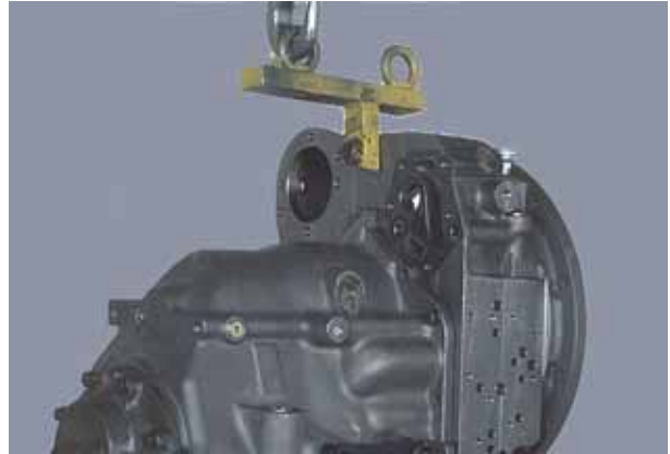
Figure 28 Support converter housing with a chain hoist. Remove remaining bolt.
