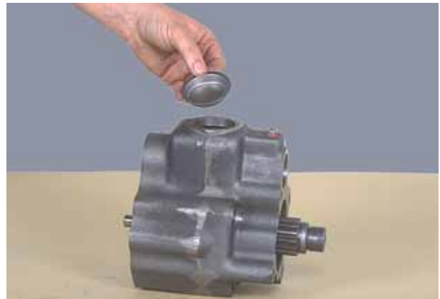
Figure 38 Apply a light coat of Loctite 577 to the outer diameter of the housing plug. Tap plug into position in housing.
