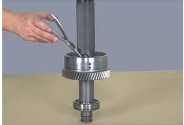
Figure 133 Compress piston return spring and spring retainer. Remove retainer ring.
