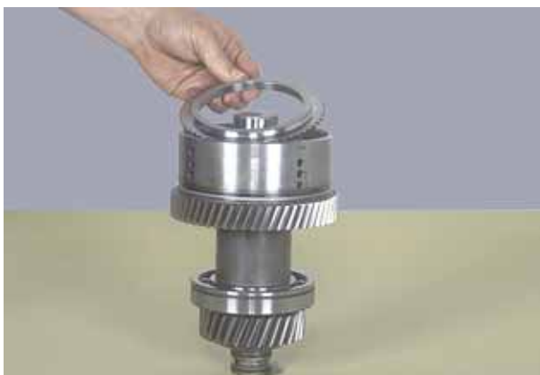
Figure 171 Install end plate.
