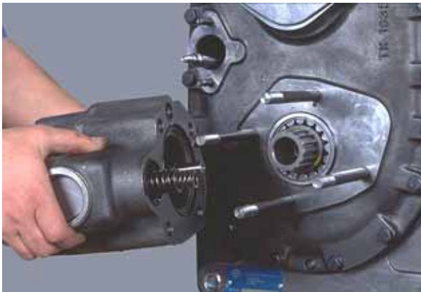
Figure 41 Use new "O"-rings on assembly. Position disconnect assembly on disconnect mounting studs. Install stud nuts and lockwashers.
