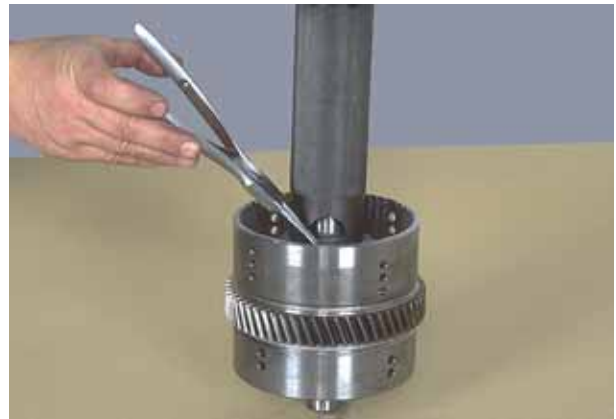
Figure 98 Compress piston return disc springs. Remove return spring retainer ring.
