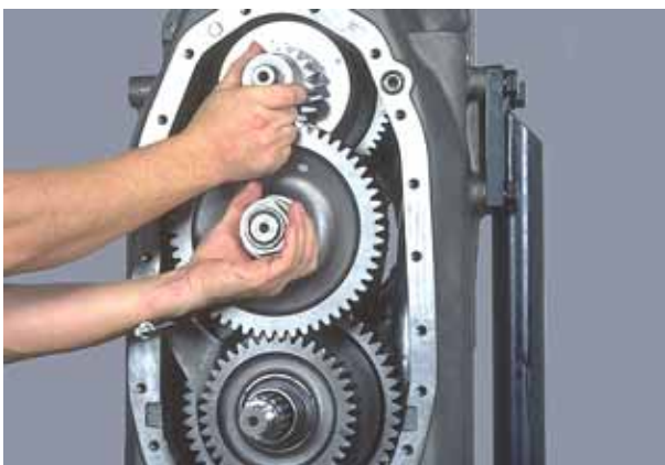
Figure 252 The low clutch (1st) and the idler shaft must be installed in the transmission case together. The help of an assistant or by replacing the transmission case on the front face may facilitate this step. Spread ears on low and idler shaft front bearing retaining ring. From the rear, tap low and idler shaft into position being sure snap rings are in full position in ring grooves.
