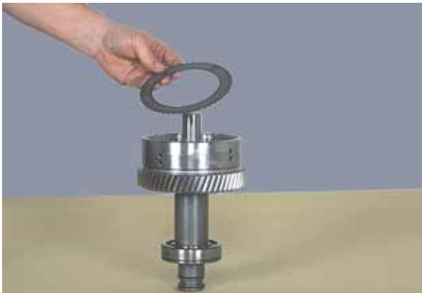
Figure 146 Install on steel disc.
