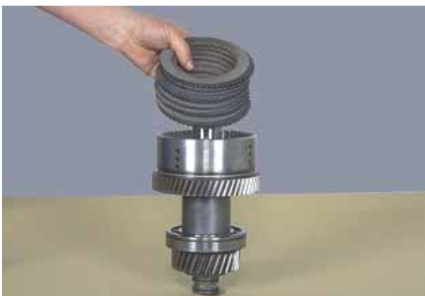
Figure 152 Remove inner and outer clutch discs.
