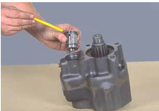
Figure 36 Position two new "O"-rings on piston bore plug. Align hole in plug with hole in housing. Install plug.
