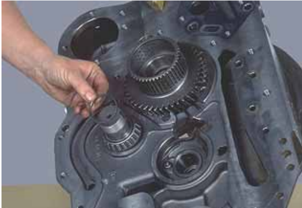
Figure 203 Position bearing spacer on shaft.
