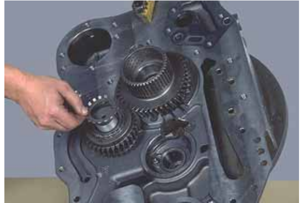
Figure 206 Install reverse idler bearing retainer nut lockplate as shown.
