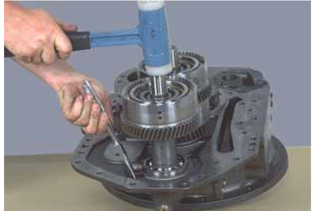
Figure 212 Spread ears on 3rd clutch front bearing locating ring. Tap clutch assembly into converter housing. Align the snap ring groove in the front bearing with the snap ring in the housing, being certain bearing snap ring is in full position in snap ring groove.
