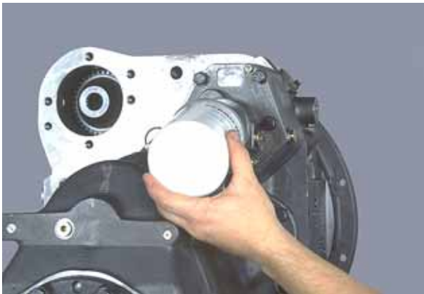
Figure 287 Install new oil filter. Tighten 20 to 25 ft. lbs torque (27.1 - 33.9 N.m.). NOTE: it is recommended that the filter cartridge be changed after 100 hours of operation on new and rebuilt or repaired units.
