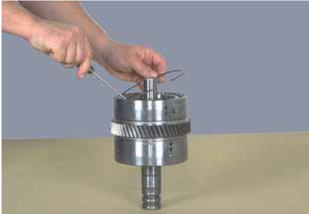
Figure 101 Remove end plate retainer ring.
