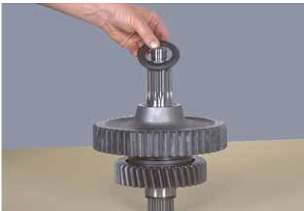
Figure 17 Install low range gear thrust washer.
