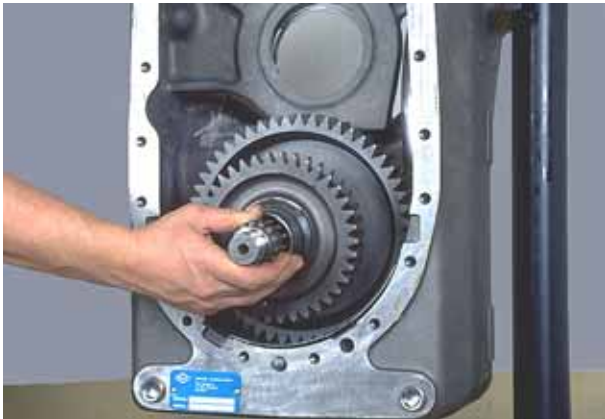
Figure 56 Remove output shaft assembly from housing.
