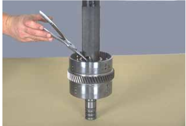
Figure 104 Compress piston return spring. Remove retainer ring.
