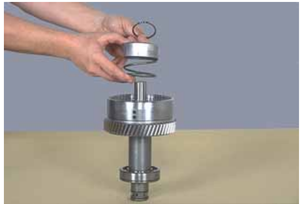
Figure 134 Remove return spring, spring retainer and retainer ring.
