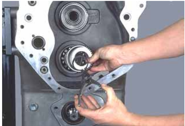
Figure 47 Remove 3rd clutch disc and retaining ring.
