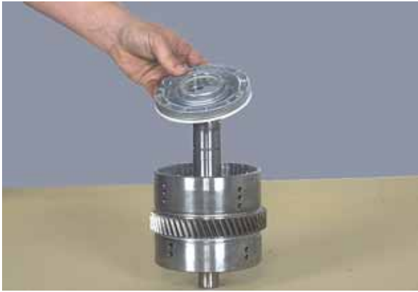
Figure 100 Remove clutch piston.2nd being disassembled.
