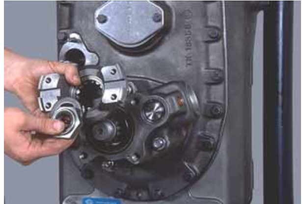
Figure 43 Install output flange "O"-ring, washer and flange nut.
