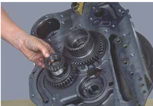
Figure 205 Install taper bearing on shaft with large diameter of taper up.
