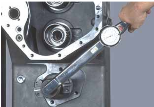
Figure 276 Block flange to prevent turning. Tighten flange nut 200 – 250 lbs. ft. (371.2 – 339.0 Nm.).
