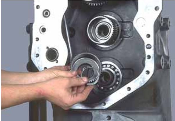
Figure 274 Install 3rd clutch disc hub and retaining ring.
