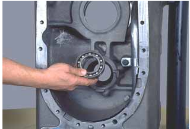
Figure 58 From the front tap output shaft bearing from housing.
