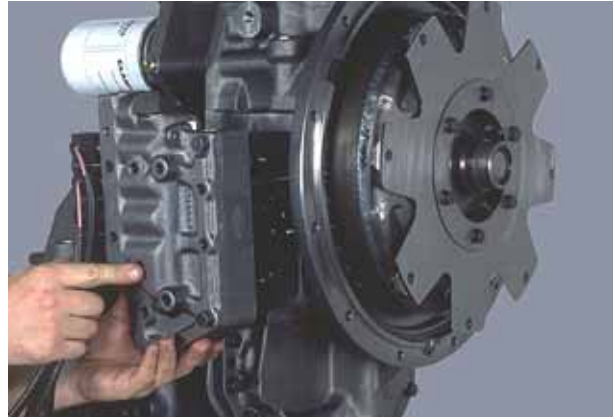
Figure 301 Position control valve assembly on aligning studs.
