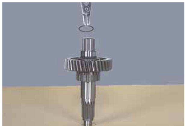
Figure 6 Remove bearing inner race retaining ring.
