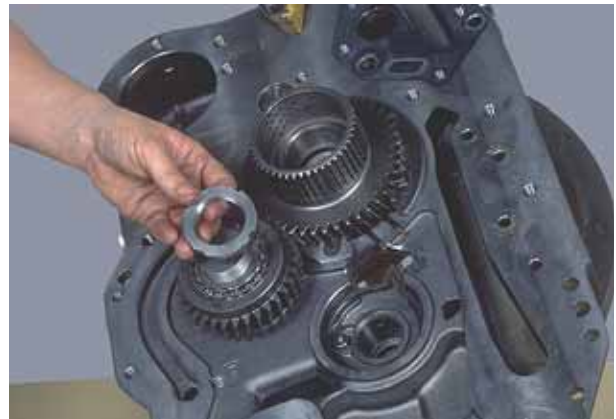
Figure 207 Install reverse idler bearing nut with chamfer down.
