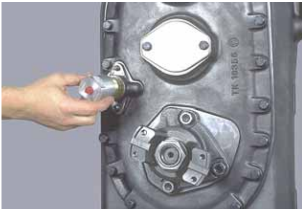
Figure 269 Install cap and "O"-ring on cylinder tube. Tighten cap securely.
