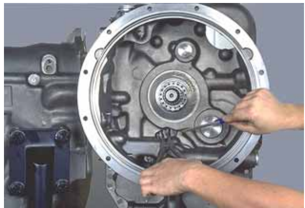
Figure 30 Using spreading type snap ring pliers, spread ears on the reverse clutch front bearing retaining ring.
