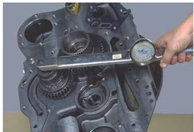
Figure 208 Tighten nut 200 to 250 ft. lbs. Torque (271.2 – 338.8 Nm.). Use TG 1304-54.
