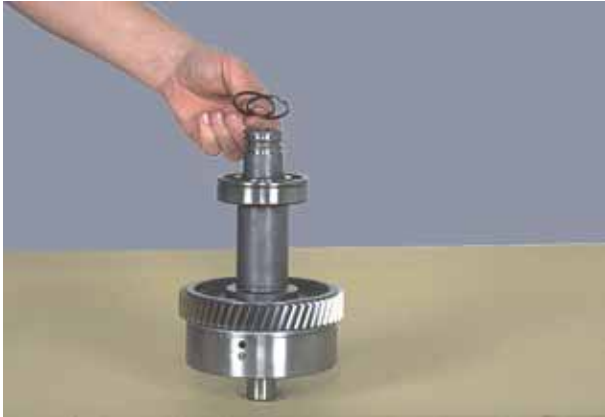
Figure 136 Remove clutch shaft piston rings.
