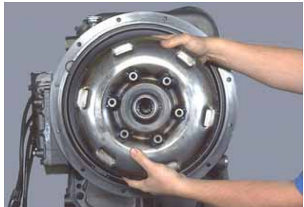
Figure 11 Remove torque converter assembly.
