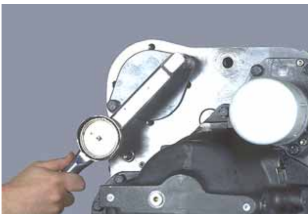
Figure 288 Install pump hole cover, news gasket, screws and lockwashers. Tighten screws to specified torque (see torque chart).
