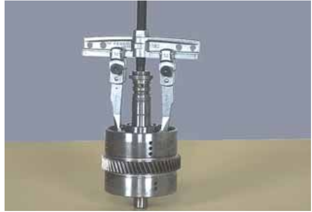
Figure 97 Remove clutch gear inner bearing.
