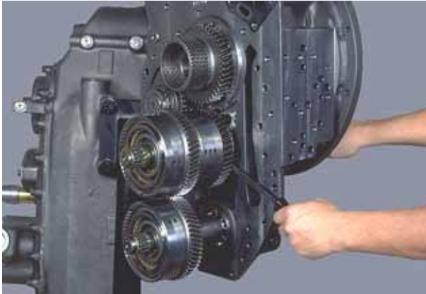
Figure 31 Holding snap ring open pry reverse and 2nd clutch assembly from converter housing.
