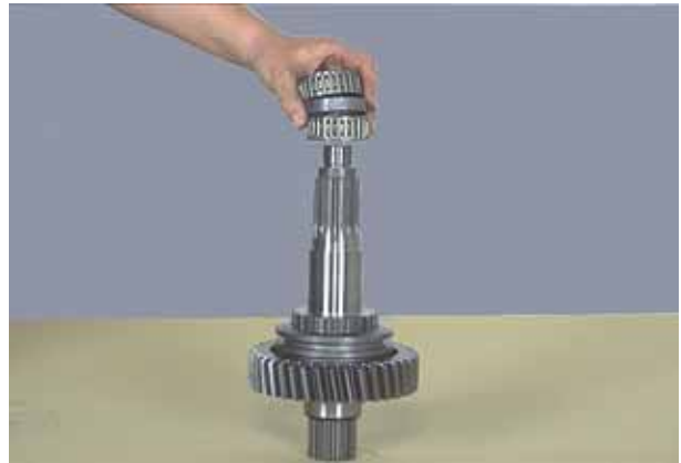
Figure 4 Remove low range gear bearings and spacer.
