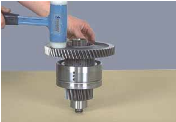
Figure 84 Install clutch driven gear and hub into clutch drum. Align splines on clutch hub with internal teeth of friction discs. Tap gear into position. Do not force this operation. Gear splines must be in full position with internal teeth of all friction discs.
