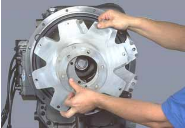
Figure 7 Remove drive plate and backing ring.
