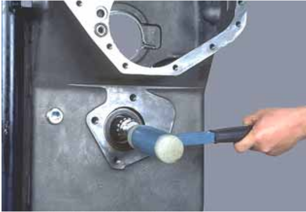
Figure 55 From the front tap output shaft from the front bearing, bearing remains in transmission case.
