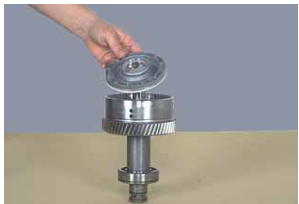
Figure 135 Remove clutch piston.
