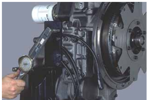
Figure 303 Install protection cover, screws and lockwashers. Tighten screws to specified torque (see torque chart).
