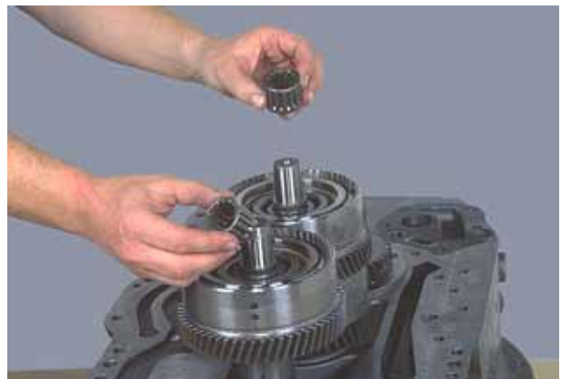
Figure 213 Position the 2nd speed clutch shaft and 3rd speed clutch pilot bearings on clutch shaft, a light coat of good quality grease will hold bearing in position on shaft.
