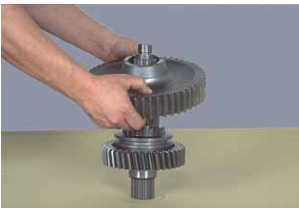
Figure 3 Remove low range gear.
