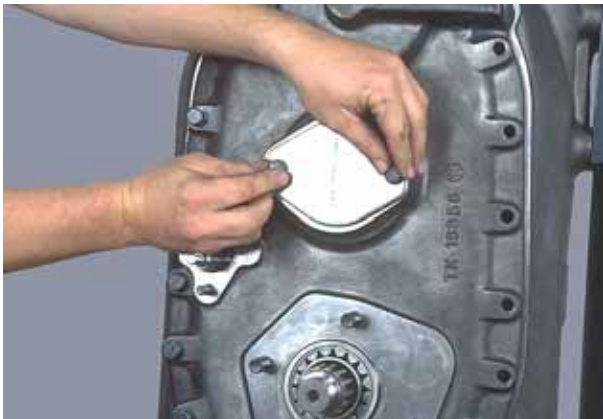
Figure 257 Install pump hole cover, gasket, screws and lockwasher.
