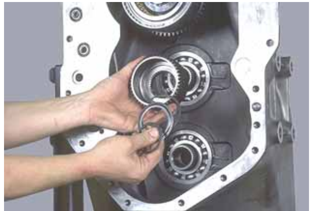
Figure 272 Install 2nd disc hub, hub retaining ring, retaining ring retainer and retainer locating ring. See figure 273.
