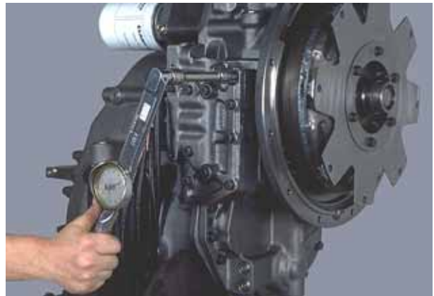
Figure 302 Install control valve to converter housing screws and lockwashers, tighten screws to specified torque (see torque chart).
