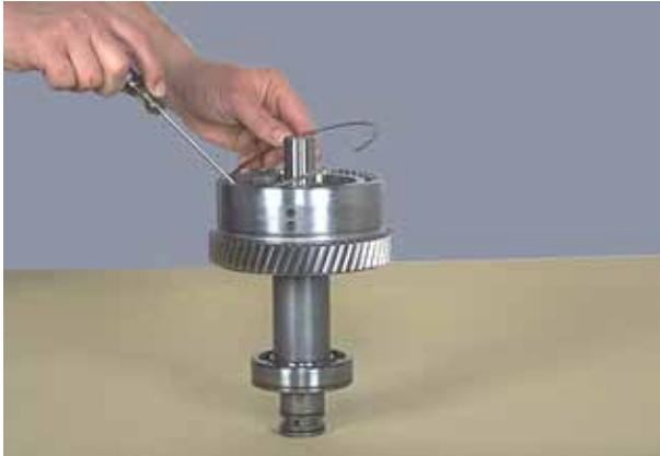
Figure 130 Remove end plate retainer ring.
