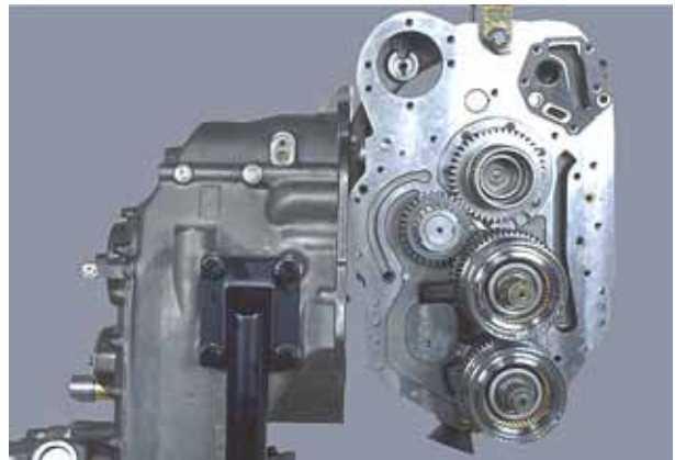
Figure 29 Separate converter housing from transmission case assembly. NOTE: Reverse and 2nd and 3rd clutch will remain in converter housing.
