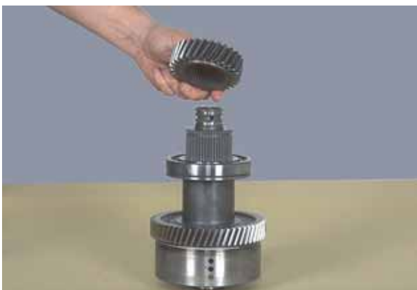
Figure 158 Remove 1st drive gear.
