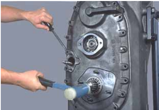
Figure 44 Using pry slots provided, pry cover from transmission housing. Using a soft hammer tap on idler and output shafts to prevent cover from binding.
