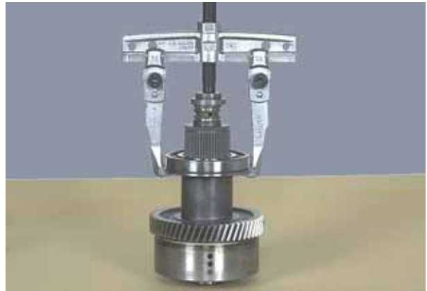
Figure 159 Remove forward clutch shaft rear bearing.
