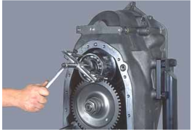
Figure 46 Remove low clutch rear bearing.
