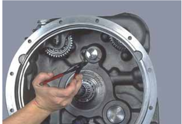
Figure 289 Install idler gear bearing retaining ring.
