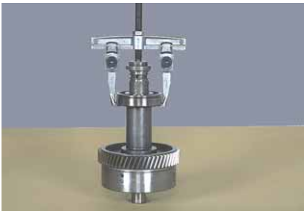
Figure 138 Remove clutch shaft front bearing.
