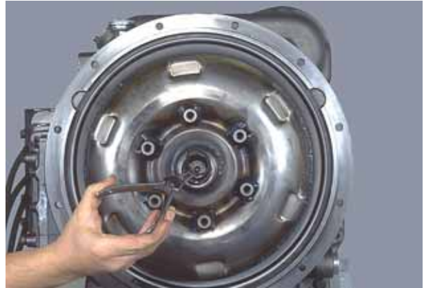
Figure 10 Through bore plug hole, remove turbine retaining ring.
