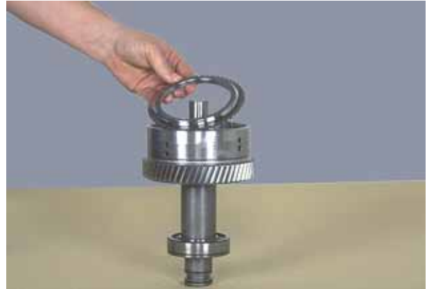
Figure 148 Install end plate.
