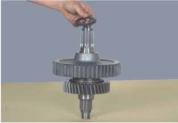
Figure 243 Install low range gear thrust washer.
