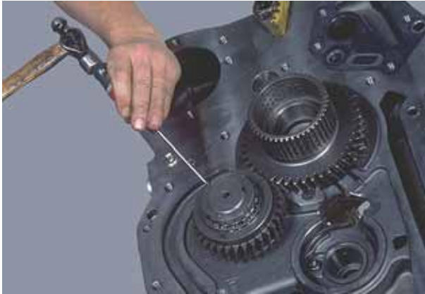
Figure 209 Bend over tag of lock plate that aligns with one of the slots of the lock nut, to secure it (See figure 210).
