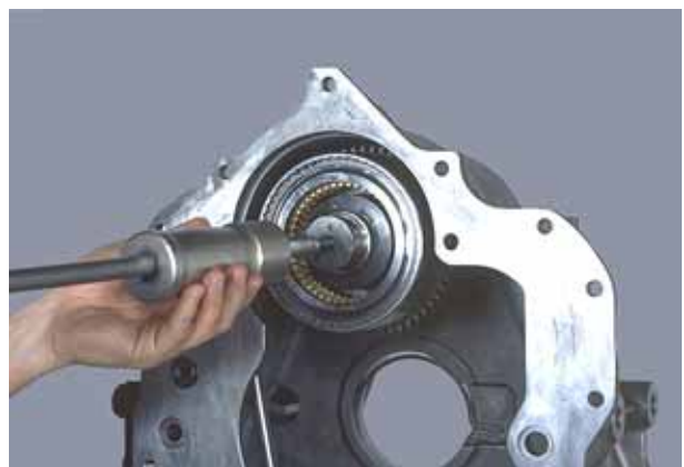
Figure 60 While holding locating ring open, use a hammer puller to remove forward shaft and clutch assembly. Internal THD M10 x 1.5 deep 15mm.
