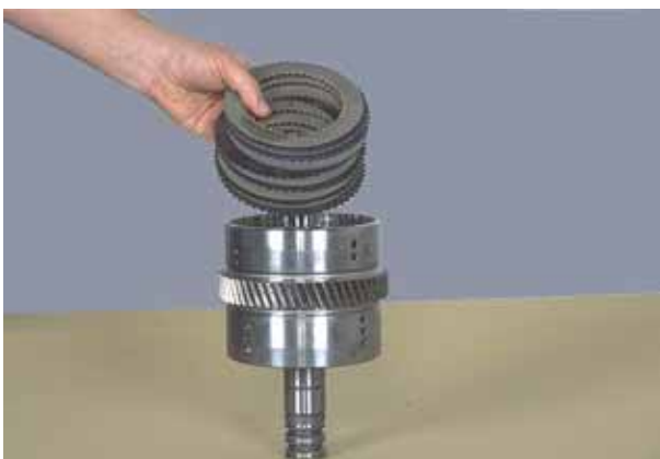
Figure 103 Remove inner and outer clutch discs.
