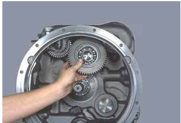
Figure 290 Position pump idler gear and bearing in stab shaft.
