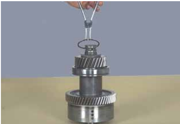
Figure 157 Remove 1st drive gear retaining ring.
