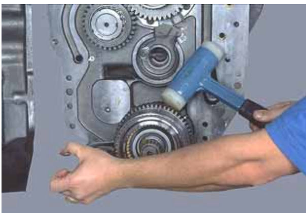
Figure 33 Holding snap ring open tap 3rd clutch from converter housing.
