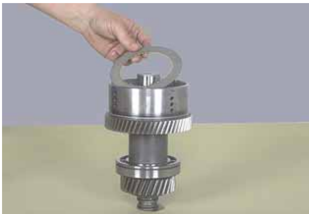
Figure 170 Install one friction disc. Alternate steel and friction discs, until the proper amount of discs are installed. First disc next to the piston in steel, last disc installed is a friction disc.
