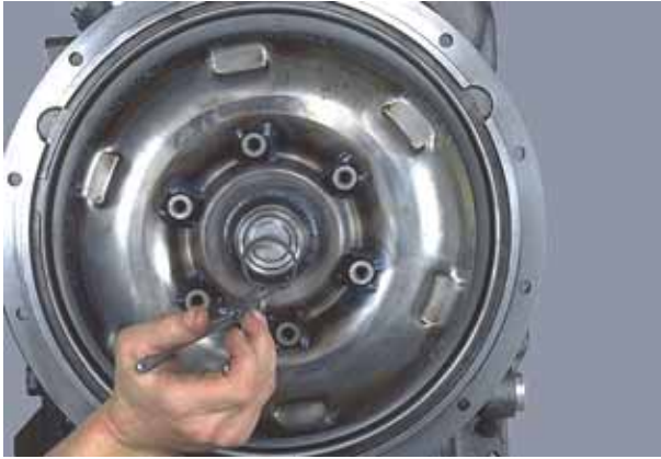
Figure 298 Install bore plug retaining ring.
