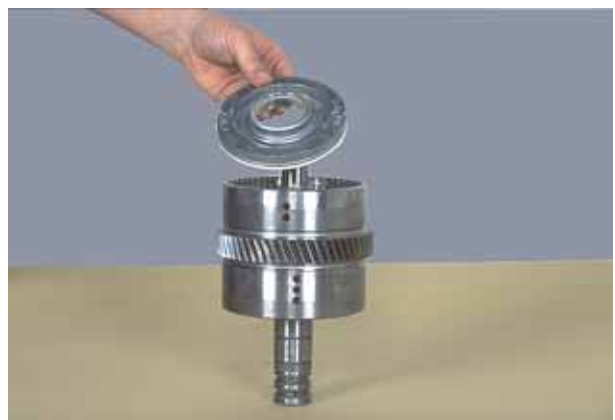
Figure 106 Remove clutch piston. Reverse and 2nd clutch reassembly 2nd being assembled.
