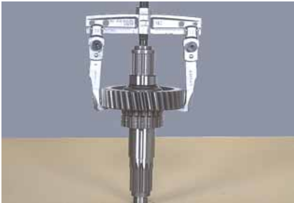
Figure 7 Remove high range gear, gear thrust washer, bearing spacer and bearing inner race.
