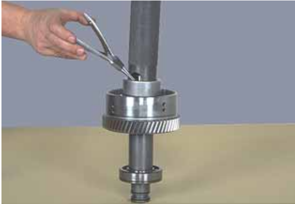
Figure 145 Compress return spring and install retainer ring.
