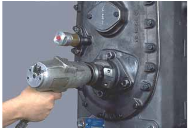
Figure 35 Remove output shaft rear flange nut, washer, "O"-ring and flange.
