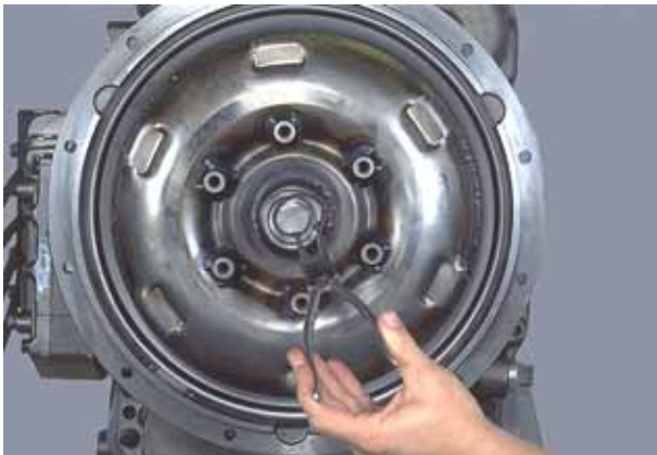
Figure 8 Remove impeller cover bore plug retainer ring.
