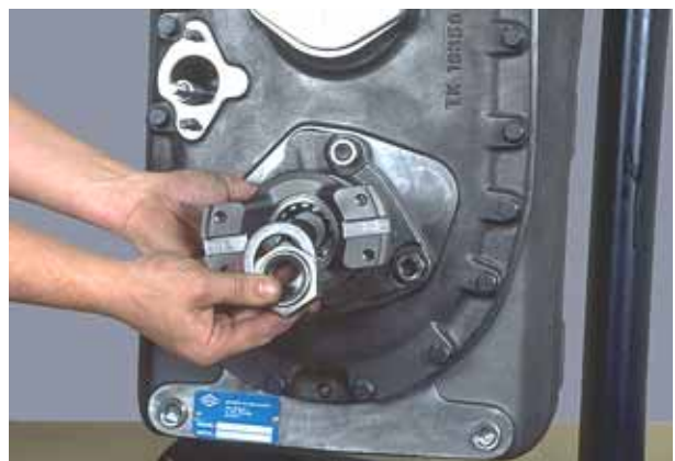
Figure 261 Install output flange, "O"-ring, washer and nut.
