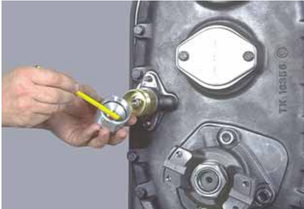
Figure 268 Position new cylinder end cap "O"-ring into end cap.
