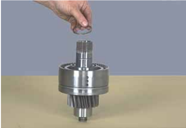
Figure 83 Install low speed gear bearing spacer.
