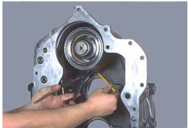
Figure 59 Open ears on forward shaft rear bearing locating ring.
