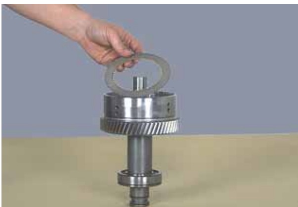
Figure 147 Install one friction disc. Alternate steel and friction discs until the proper amount of discs are installed. First disc next to the piston is steel, last disc installed is a friction disc.
