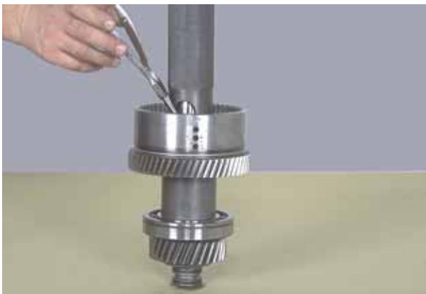
Figure 167 Position spring nap ring. Compress spring. Install snap ring.
