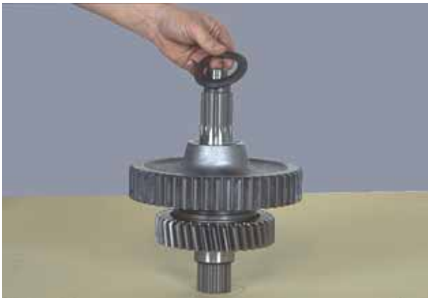
Figure 2 Remove low range gear thrust washer.
