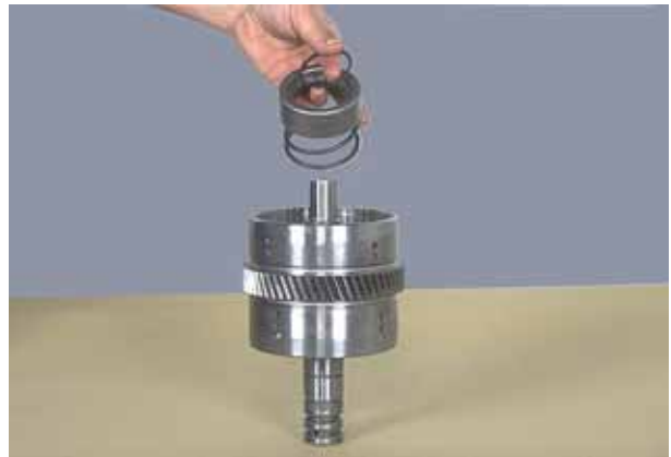
Figure 105 Remove return spring, spring retainer and retainer ring.
