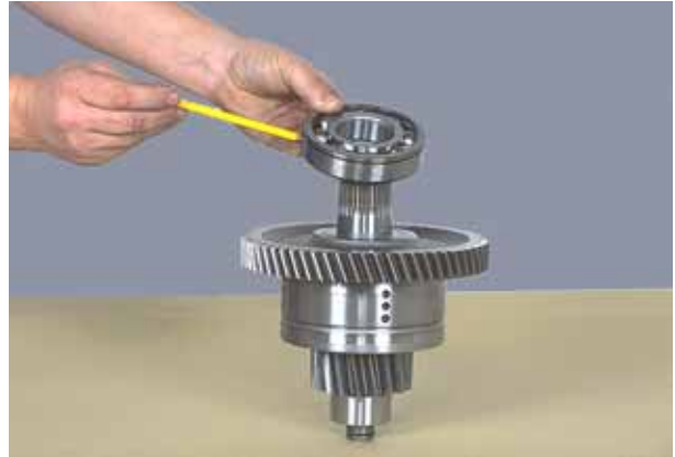
Figure 86 Install low shaft front bearing with bearing groove up.
