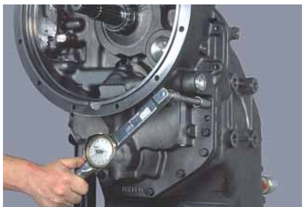
Figure 279 Tighten cap screws to specified torque (see torque chart).
