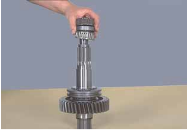
Figure 15 Install low range gear bearings and spacer.
