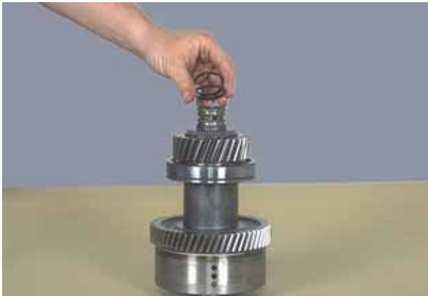
Figure 156 Remove forward clutch shaft piston rings.
