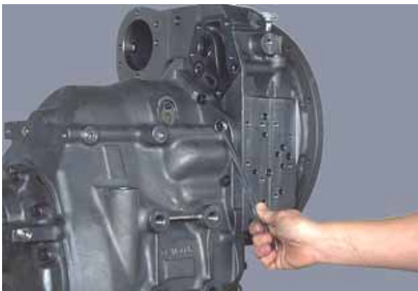
Figure 27 Remove all bolts but one securing transmission to converter housing.
