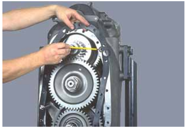
Figure 254 Position new gasket and "O"-ring on rear of transmission housing. A thin coat of chassis grease will hold the gasket and "O"-ring in place.
