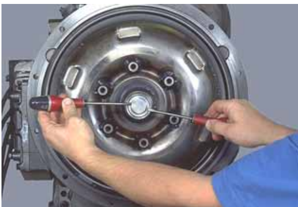
Figure 9 Using two small screw drivers as shown, remove plug.
