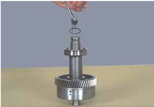
Figure 137 Remove clutch shaft front bearing retainer ring.
