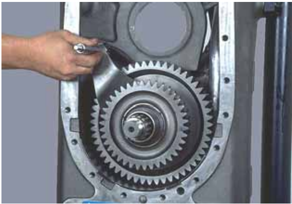
Figure 251 Install shaft fork and rod as an assembly on shift hub.
