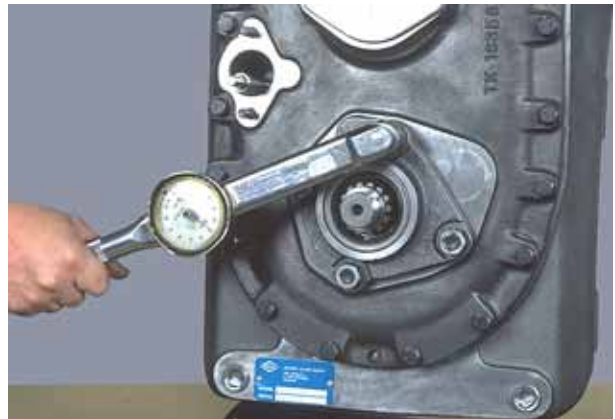
Figure 260 Install lockwashers and stud nuts. Tighten nuts to specified torque (see torque chart).
