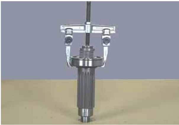
Figure 221 Remove idler shaft front bearing.
