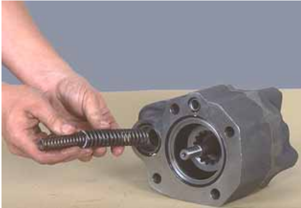
Figure 40 Insert the actuator piston inner and outer return springs in piston.
