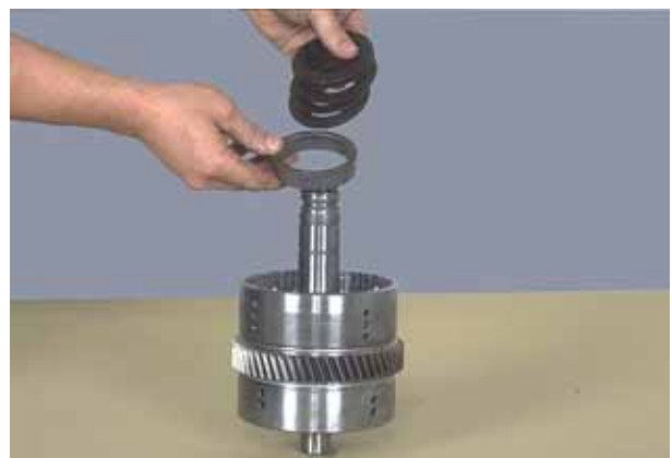
Figure 99 Remove piston return disc springs and piston spacer. See note in figure 68.
