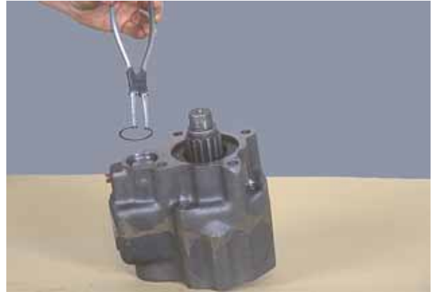
Figure 37 Secure bore plug with retaining ring.
