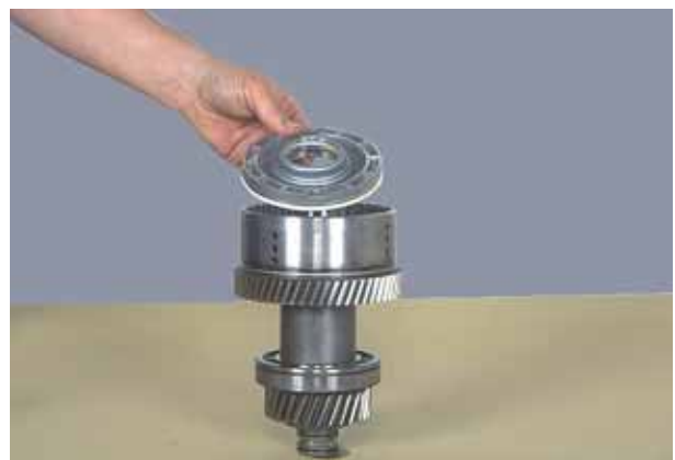
Figure 155 Remove clutch piston.
