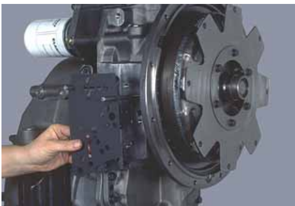
Figure 300 To install control valve assembly it is recommended two aligning studs be used to position new control valve gasket.
