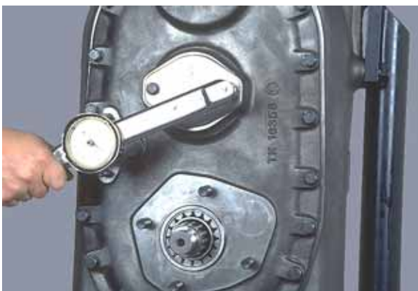
Figure 258 Tighten screws to specified torque (see torque chart).
