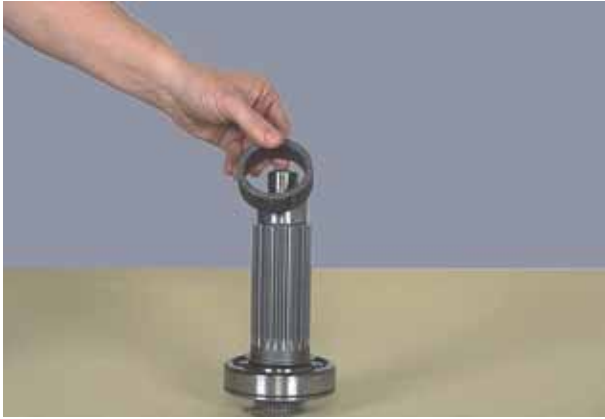
Figure 220 Remove idler shaft gear spacer.
