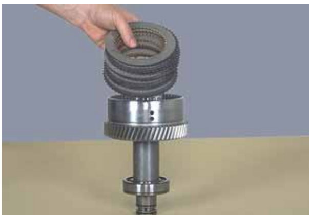
Figure 132 Remove inner and outer discs.
