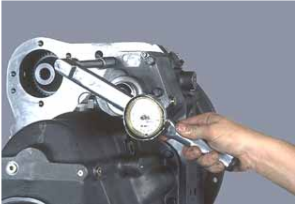
Figure 286 Install cap screws and lockwashers: tighten screws to specified torque (see torque chart).
