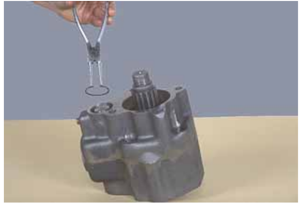
Figure 21 Remove piston bore plug retainer ring.
