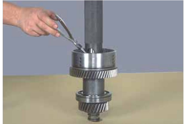
Figure 153 Compress piston return disc springs. Return spring retainer ring.
