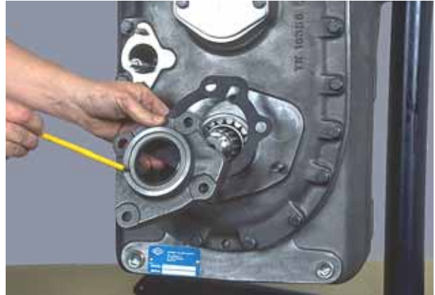
Figure 259 Press new seal in bearing cap with lip of seal toward bearing side of bearing cap. Position new gasket on bearing cap. NOTE: some units will have "O"-rings between the cap and the cover.
