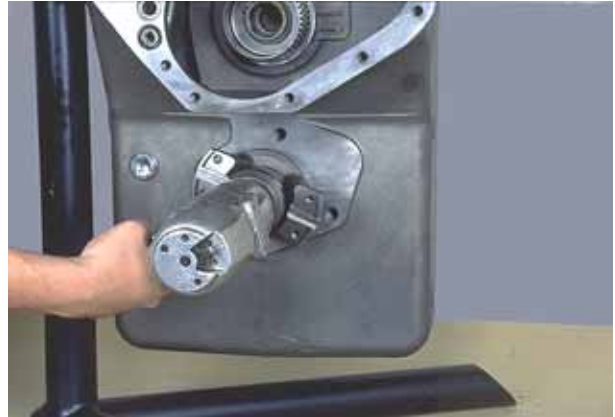
Figure 34 Remove output shaft front flange nut, washer, "O"-ring and flange.
