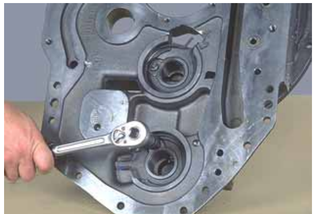
Figure 184 Remove oil sealing ring sleeve retainer and washer. Remove sleeve lock.
