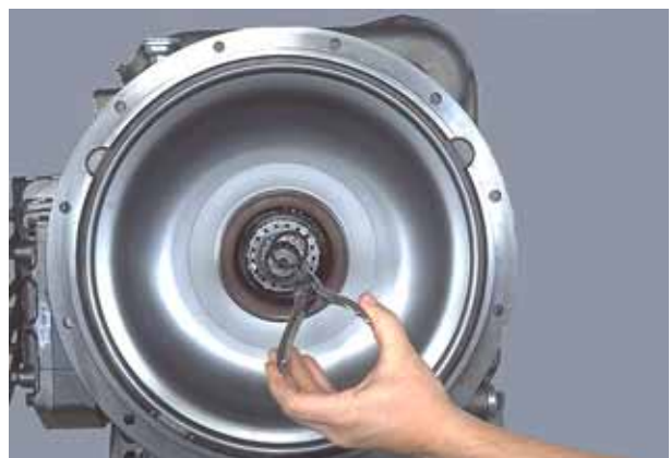
Figure 12 Remove turbine locating ring.
