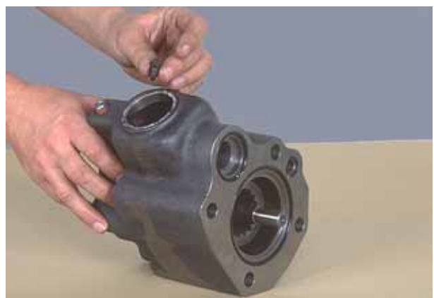
Figure 23 Remove the shift fork lock screw.
