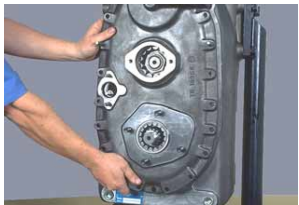
Figure 255 Install rear cover and bearing outer races as an assembly. NOTE: two aligning studs facilitate cover to housing assembly. Tap cover bores in place aligning shaft bearings with bearing bores. Use caution as not to damage low clutch shaft sealing ring. Remove aligning studs and install cover bolts and lockwashers.
