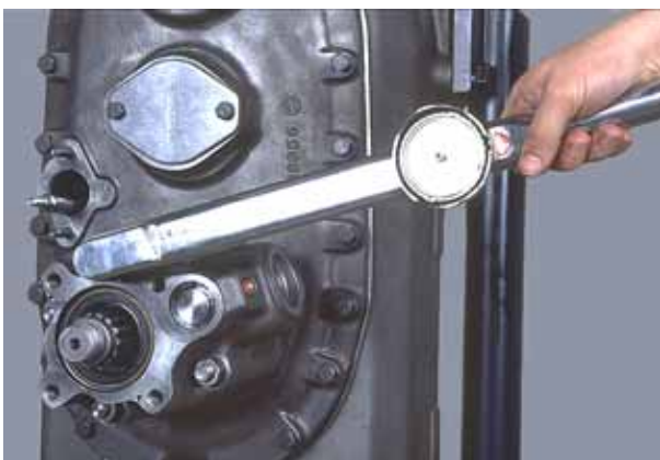
Figure 42 The actuator piston springs must be compressed against the rear cover to start the stud nuts and lockwasher. Tighten stud nuts to specified torque (see torque chart).
