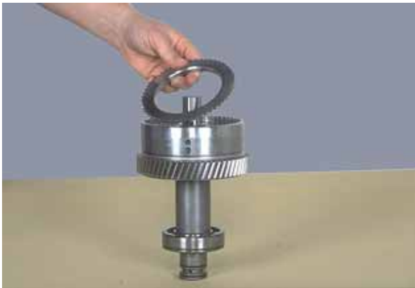
Figure 131 Remove end plate.
