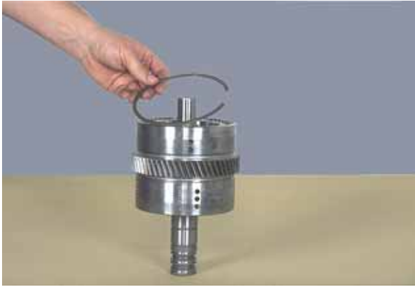
Figure 113 Install end plate and retainer ring.
