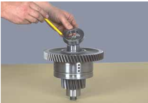
Figure 85 Install low speed gear outer bearing. NOTE: outer bearing has a shield in it, this shield must be up.
