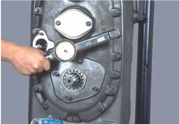
Figure 256 Tighten rear cover screws to specified torque (see torque chart).
