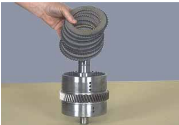
Figure 96 Remove inner and outer discs.
