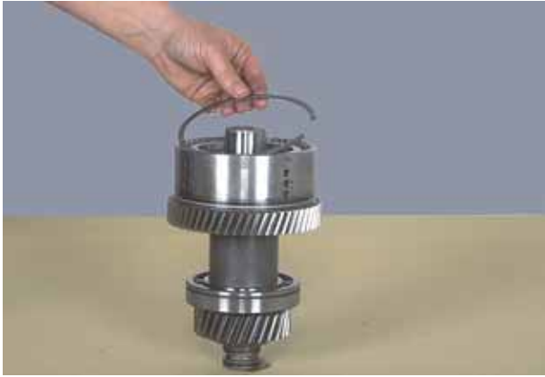
Figure 172 Install end plate retainer ring.
