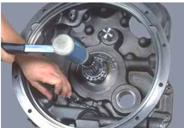
Figure 181 Using spreader type pliers spread ears on the turbine shaft bearing snap ring. Tap turbine shaft and bearing from converter housing.
