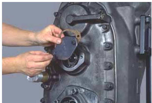
Figure 36 Remove pump hole cover, cover gasket screws and lockwashers.
