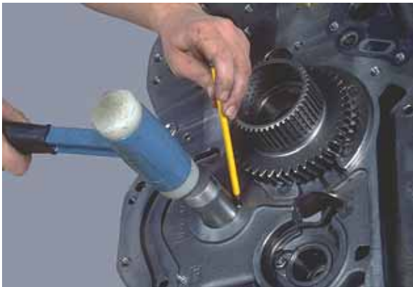
Figure 180 Remove idler shaft , use caution as not to lose shaft lock ball.
