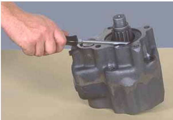
Figure 19 The output oil seal must be destroyed by using a punch to drive through the oil seal housing and picking the oil seal out of the disconnect housing.
