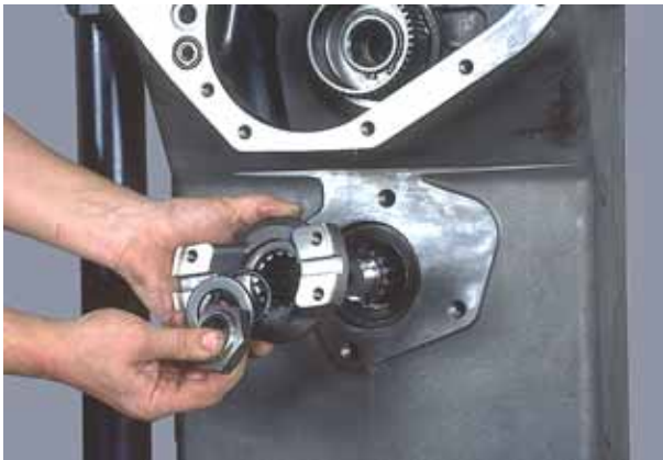
Figure 275 Install front output flange , "O"-ring, washer and flange nut.
