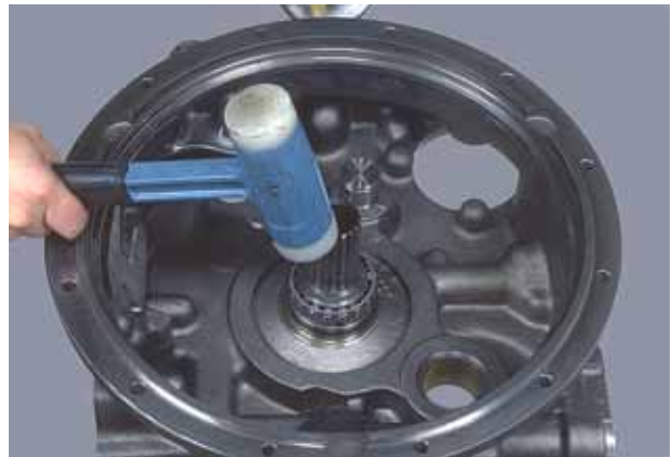
Figure 183 Tap stator support from converter housing.
