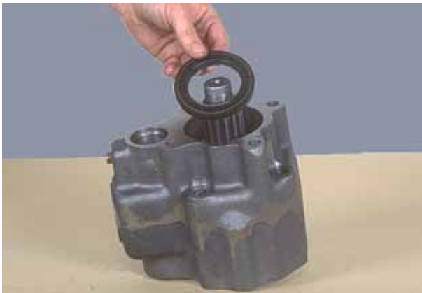
Figure 35 Press seal in disconnect housing with lip of seal in.
