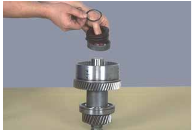
Figure 154 Remove piston return disc springs and piston spacer. See note in figure 68.
