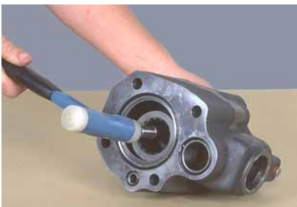
Figure 26 Tap disconnect shaft and bearing from housing.
