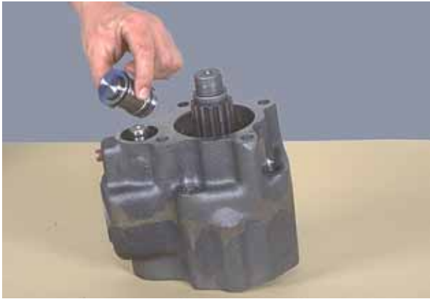
Figure 24 Remove disconnect housing plug.
