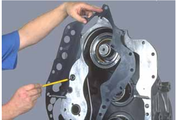
Figure 277 Position new "O"-ring and gasket on front of transmission housing. A light coat of chassis grease will hold "O"-ring and gasket in place.
