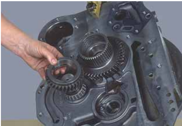
Figure 204 Position idler gear on bearing with hub of gear up.
