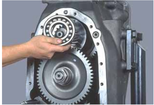
Figure 253 Install low clutch shaft rear bearing.
