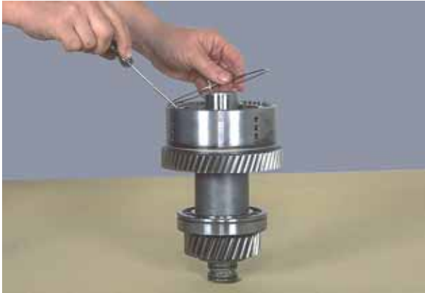
Figure 150 Remove end plate retainer ring.
