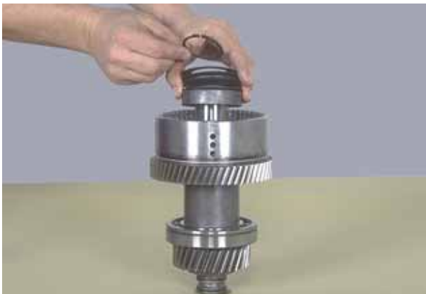
Figure 166 Position spring spacer and piston return springs. First spring with large diameter toward spacer, see figure 168. Alternate five (5) springs: see note in figure 68.
