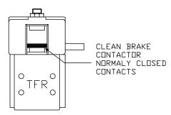
It could be necessary to replace the contactor.
