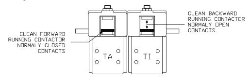
It could be neccessary to change both contactors.
