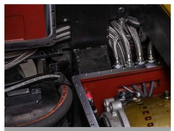
**FLEXIBLE CONDUIT (FC) CABLES** house regular cabling, which is sealed to ensure safe use in an EX-rated environment. The FC Cable provides flexibility and space saving.
